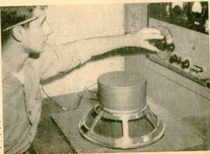
11 In the final stages of assembly, voice-coil leads are brought from spider to speaker cone. They are twisted into pigtails to prevent the damping of the cone as well as lead breakage.
