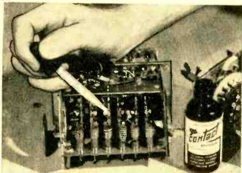
A few drops of the chemical will clean and restore the switch contacts in this tuner.
