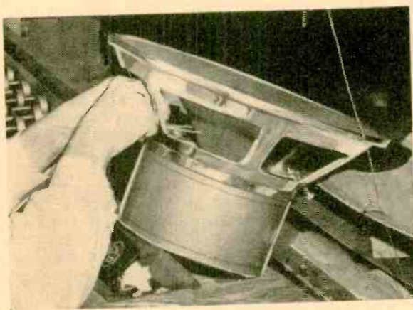
11 In the final stages of assembly, voice-coil leads are brought from spider to speaker cone. They are twisted into pigtails to prevent the damping of the cone as well as lead breakage.
