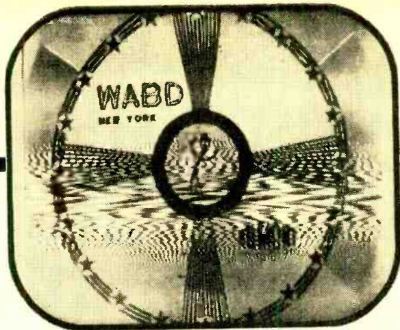
Fig. 1. Example of TV interference cured by inserting one of the filters described in this article.
