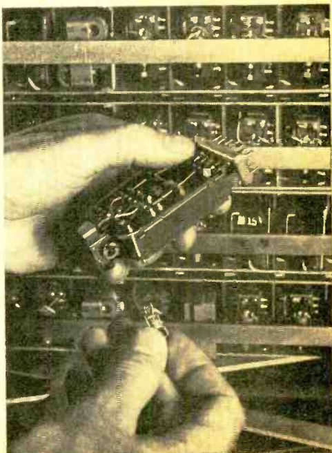
Transistor is inserted into one of TRADIC's "memory" packages. These units store information until entire problem is solved.
