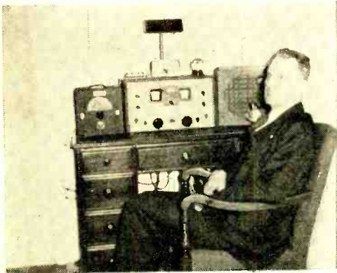
The SWL receiving station of Charles Sutton, Toledo, Ohio, illustrates a compact arrangement of equipment. The receiver is a Hammarlund HQ-129X with a RME DB-20 preselector. A 20-meter dipole is the antenna.
