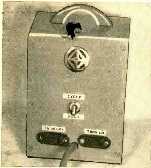
Rear view shows the ventilation cutout cover mounted above switch, S_2 . Another hole in the bottom of the box provides air circulation.
