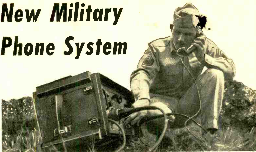
Repeater, above, amplifies conversations which may be transmitted over distance of 100 miles.
