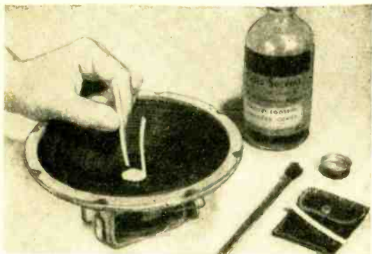
Fig. 7. After cone assembly has been loosened, insert three shims between voice coil and pole piece. Shims must be equally spaced.
