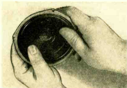
Fig. 5. Correct procedure for testing a speaker for an off-center voice coil is shown in this photo. See text for full details.
