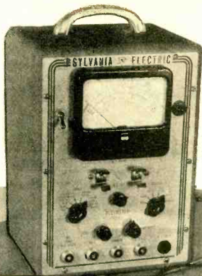
A service-type vacuum-tube voltmeter—compared in this article with the non-electronic type of multimeter.
