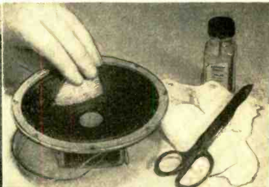
Fig. 4. Larger tears in the paper cone of the speaker may be repaired by patching over with cheesecloth held in place by cement.
