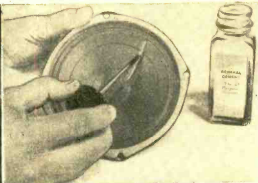
Fig. 2. Correct method for applying cement to repair an open seam on outer rim of speaker. Do not use speaker until cement has hardened.
