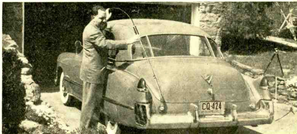
Center-loaded whip antenna on Mort Kahn's car is mounted on rear and is pulled down and tied to rain molding when car is garaged. Base spring gives flexibility.
