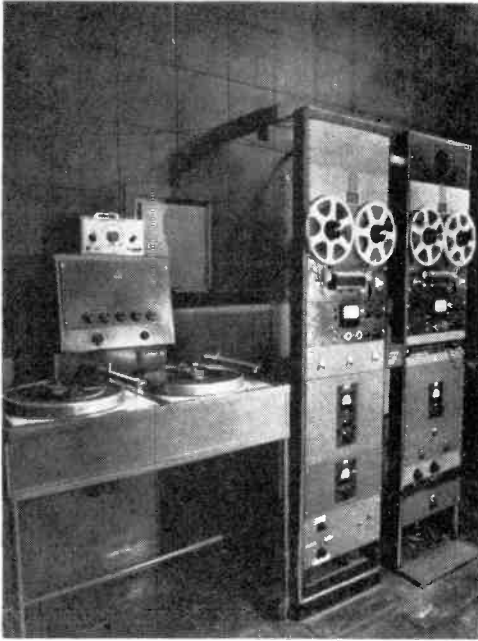
Hi-fi record and tape equipment, amplifiers, and controls are housed in soundproof room.
