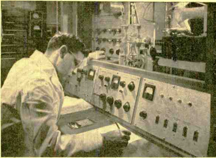
This instrument array facilitates study of radio-active medicines when the accelerator produces isotopes.
