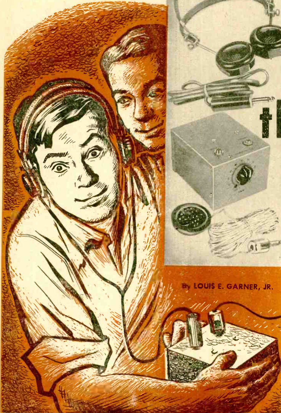
Fig. 1. The "Electronic Ear"—a microphone, an extension cable, a battery-operated amplifier, and a pair of sensitive headphones.
