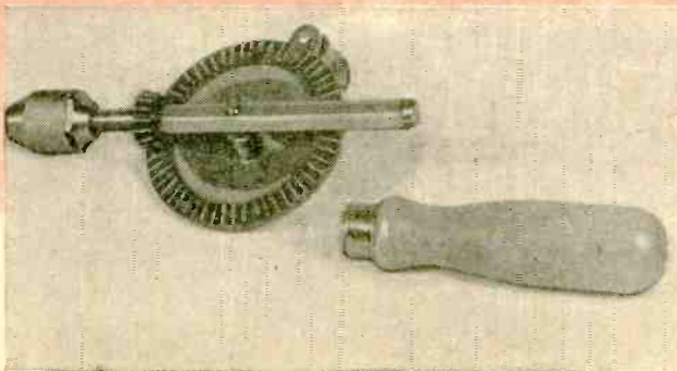
Fig. 3. The winding mechanism is simply an "egg-beater" type hand drill with the handle removed. See article on removing handle without damaging the drill.
