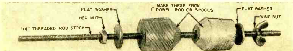
Fig. 7. Details on coil form holder. Cone-shaped rods may be turned on lathe or handmade.
