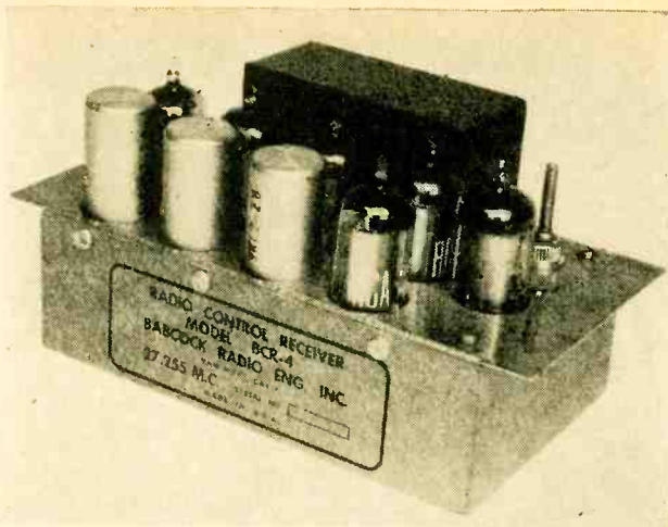
Companion radio-control receiver made by Babcock Radio Engineering, Inc., of Van Nuys. Metal "tubes" are sealed relay units.
