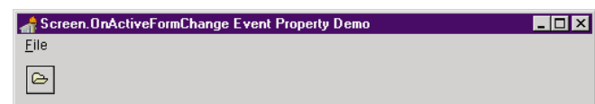
Figure 5: The ONFRMCHG.DPR project demonstrates the use of the Screen.OnActiveFormChange event handler to update the Caption property of the main form in an SDI application.
