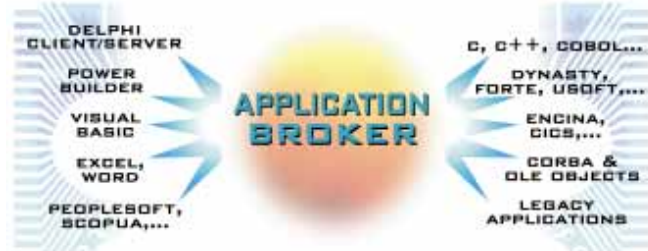
Figure 3: The Application Broker acts as an interface between client applications and server-resident business rules, regardless of their implementation.
