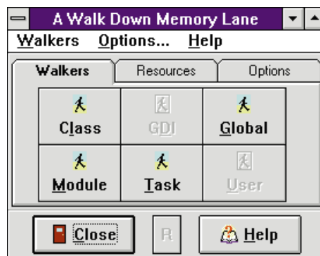
Figure 1: Walker displays information about the currently loaded modules, running tasks, the registered Windows classes, and how memory is being allocated on the Windows global heap.
