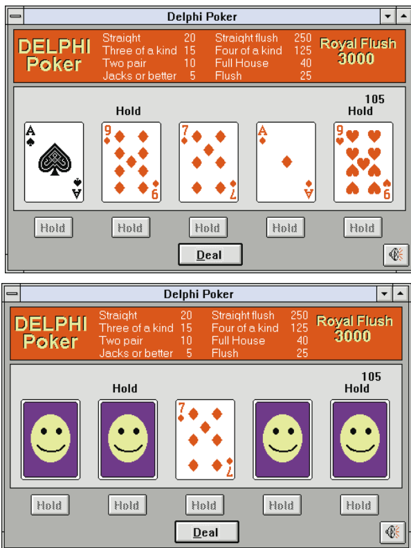
Figure 1: This video poker game was built using the TCardDeck component. The first screen shows the player held onto a pair of nines and then pressed the Deal button. When a pair of aces is added to the held cards, Delphi flashes smiles.
