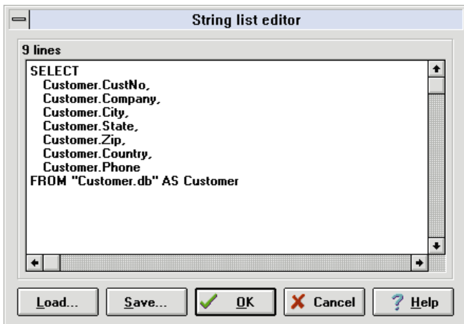
Figure 3: Using the String list editor to define the SQL property of the Query component.
