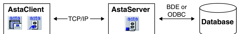
Figure 1: ASTA allows traditional two-tier practices to be used in a true three-tier environment.
