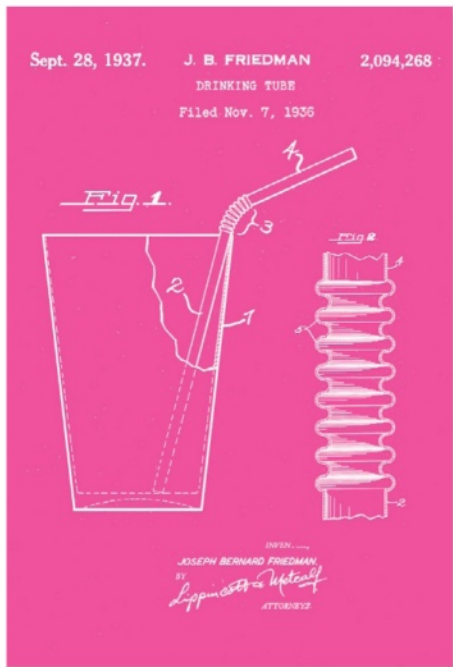
Friedman's detailed patent for the bendable straw
