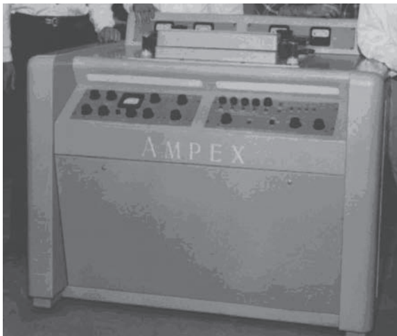
Figure 13-1 Ampex-Mark IV VTR. Courtesy of Department of Special Collections and University Archives, Stanford University Libraries.
