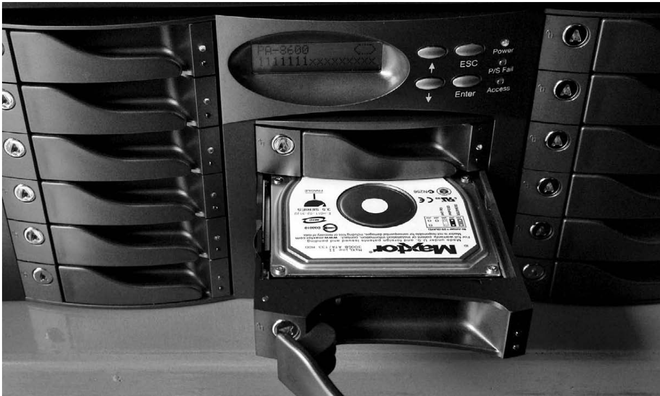
RAID works with redundancy and uses hot swappable ATA drives.
