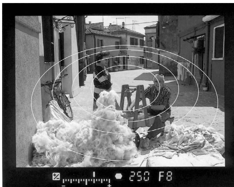
A typical light measurement display in a modern SLR camera
