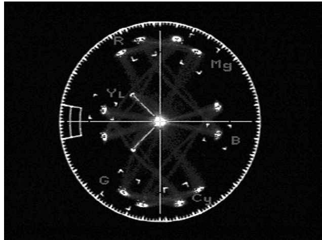
Accurate color reproduction can be checked with a vectorscope.
