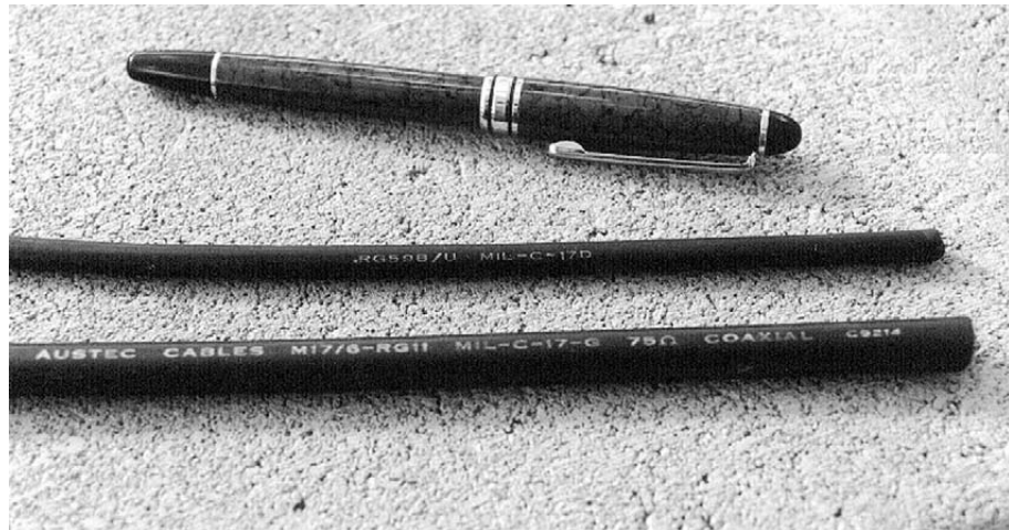
Physical size comparison between RG-59 and RG-11 coax
