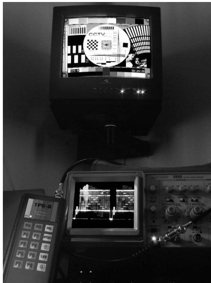
A test pattern generator signal and its waveform on an oscilloscope
