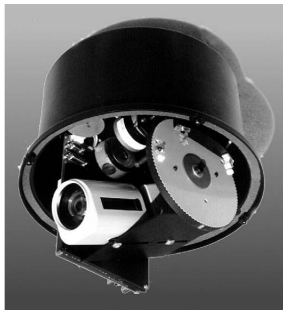
Larger pan/tilt domes accommodate a separate camera/lens combination.
