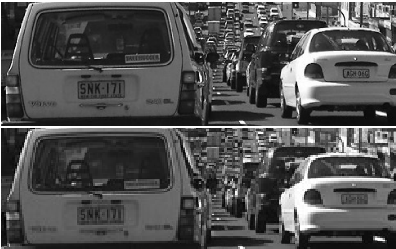
The difference between full frame 720 x 576 pixels image (above) and the same in CIF size (360 x 288) sometimes can make a difference between recognizing a license plate and not recognizing it (for example, the car on the right).
