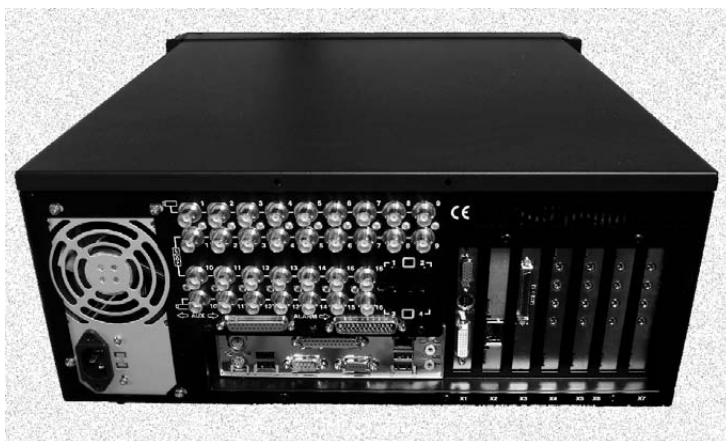
A typical DVR in CCTV has 16 camera inputs, but 18, 24, or 32 are also possible.
