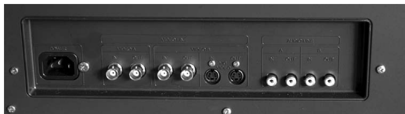
If a monitor does not have a manual switch, it means the electronics inside automatically terminate it.
