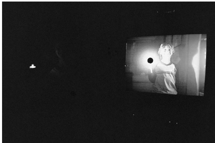
The example above shows a boy with a candle in his hand on the left-hand side, hardly noticeable by the film camera, while the CCTV camera sees it quite nicely as shown on the monitor right.
