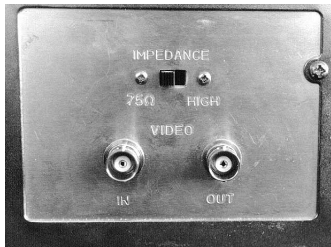
The manual impedance switch is usually at the back of monitors.
