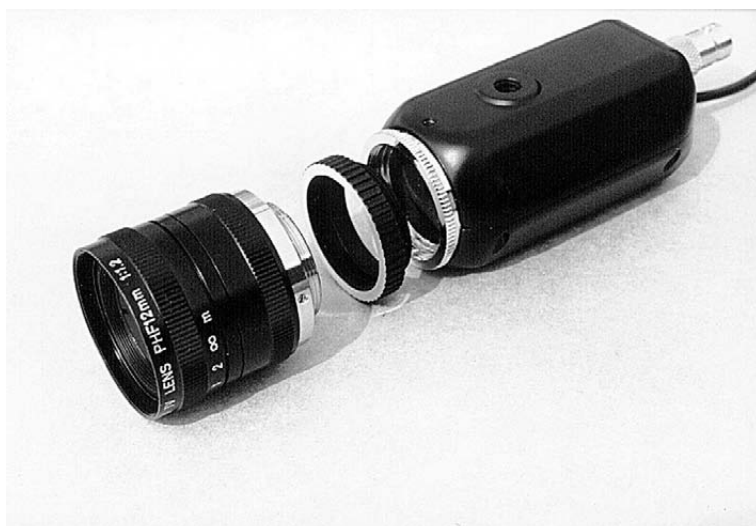
If a lens is C-mount and the camera is CS, a C/CS adaptor ring is required.
