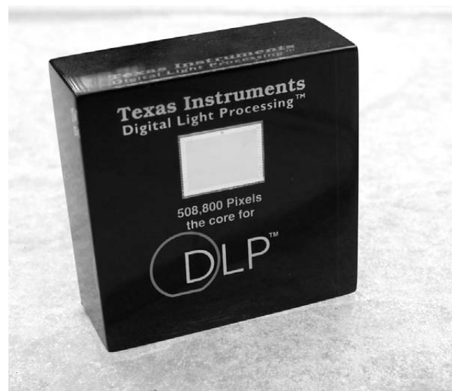
The heart of the DLP projectors, Texas Instruments' patented digital light processing chip
