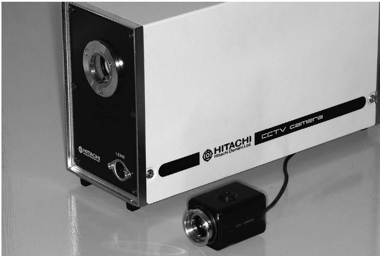
Fifteen years apart, and they do the same job (tube and CCD camera).
