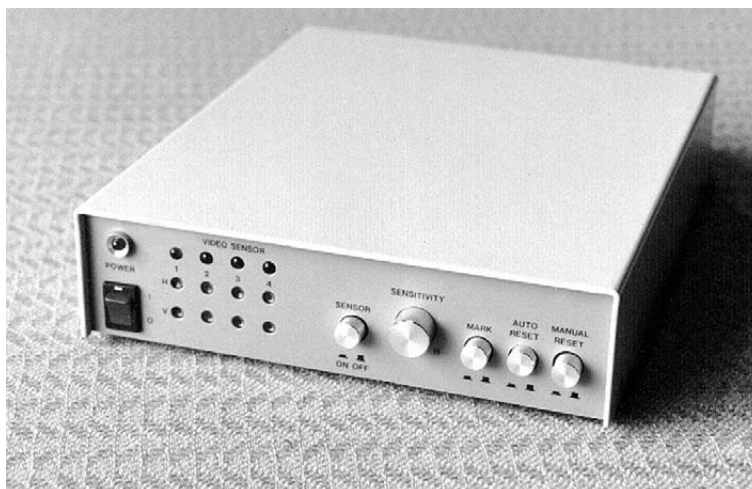
A simple non intelligent single-channel video motion detection unit
