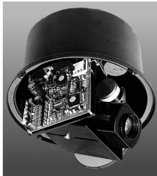
PTZ site drivers are integrated into most PTZ domes.
