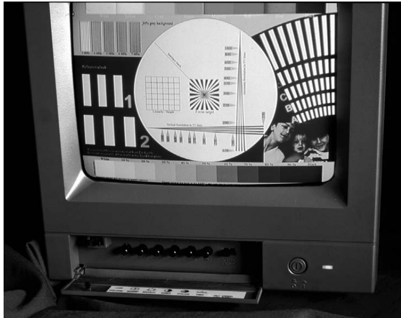
The gray scale of a test signal is used to adjust brightness and contrast to optimum setting.
