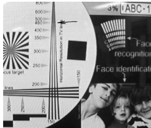
An actual photo of a camera showing around 460 TVL resolution
