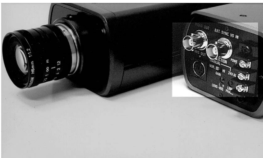
A line-locked camera (24 V AC) which also has an external vertical sync input terminal
