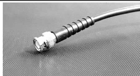
A properly terminated RG-59 coaxial cable
