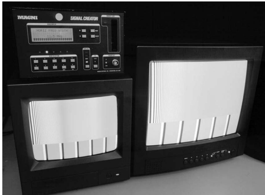
A special high-resolution sweep generator is used to check the bandwidth response of various monitors.
