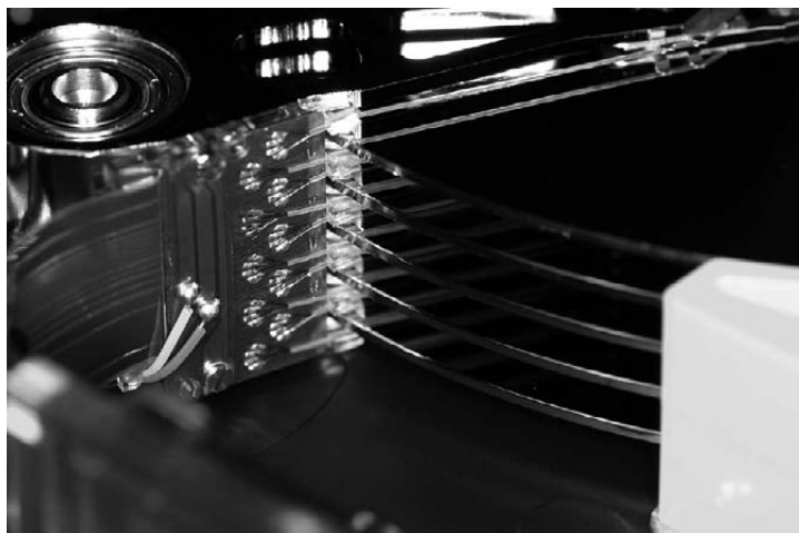
Larger hard disks usually have multiple heads and platters.
