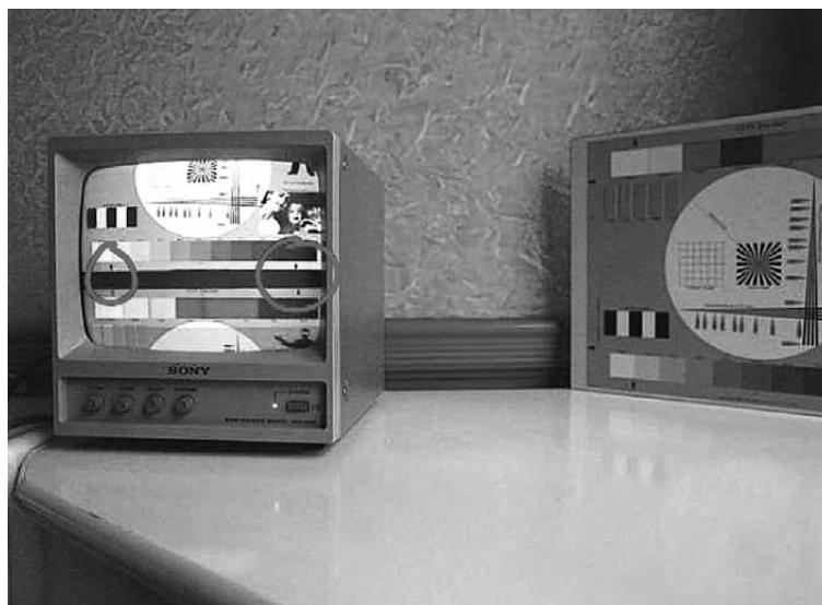
Setting up the test chart without the underscanning monitor
