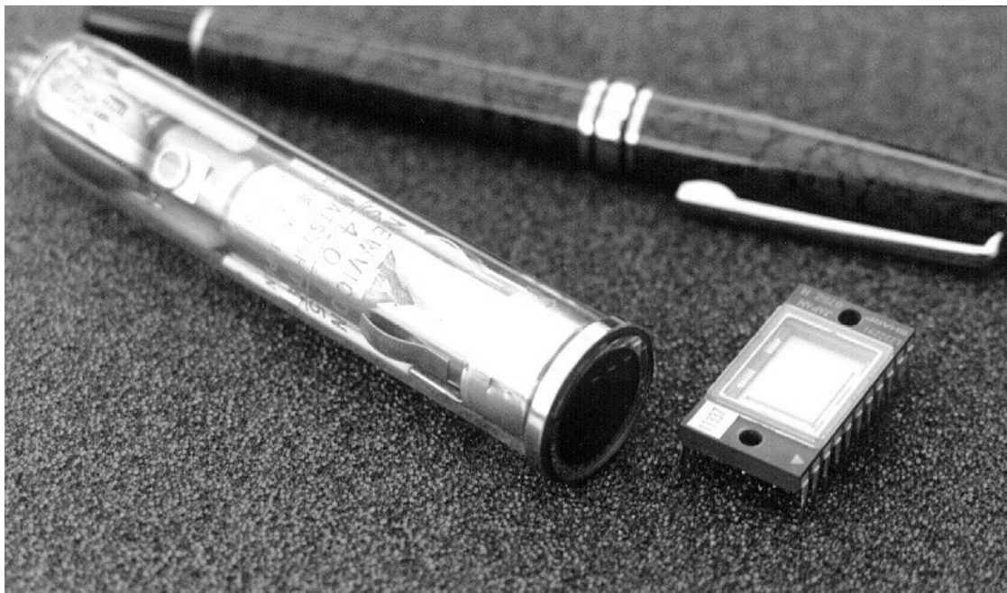
Comparison of the physical size of a tube and a CCD chip
