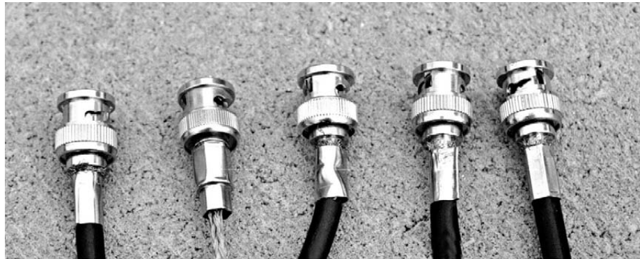
Samples of bad BNC terminations
