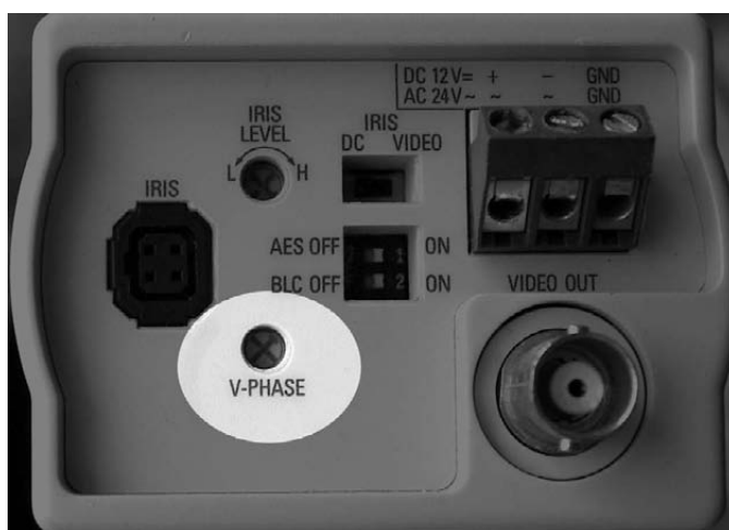
The majority of AC cameras have V-phase adjustment.
