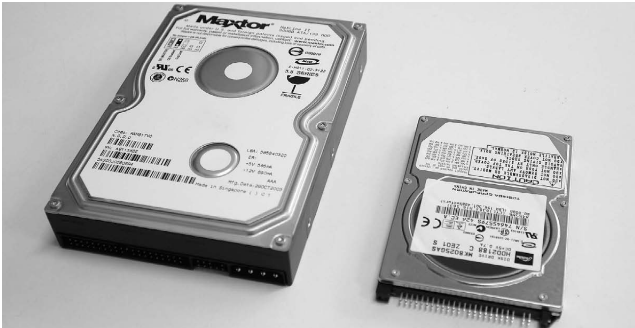
Two major sizes of hard drives: 3.5" used in desktop machines and 2.5" used in notebook computers
