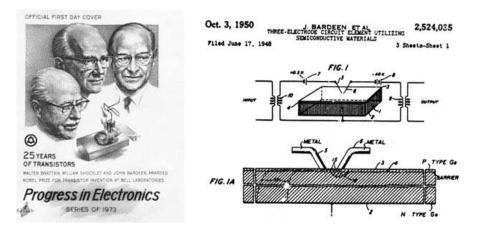
Left: The inventors of the transistor were commemorated in this U.S. Postal Service first day cover. Right: A portion of the original patent for the transistor, which was registered by and subsequently granted to the inventors from Bell Laboratories. [Cover from the collection of the author, used with permission; U.S. Patent and Trademark Office, public domain.]
