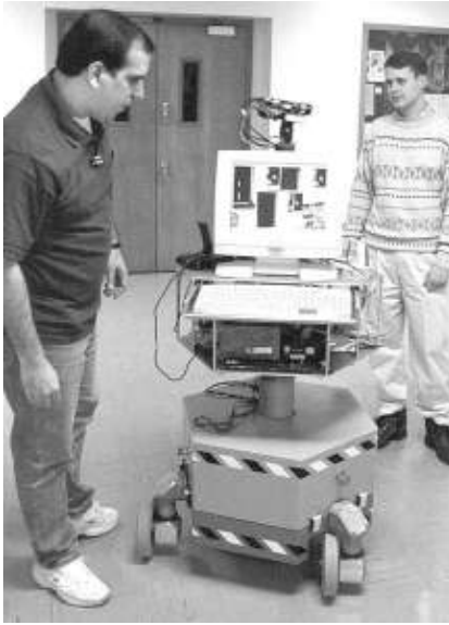
Left: Purdue Doctoral students DeSouza and Jones work with “Peter” a mobile robot equipped with a number of types of sensors. Peter can navigate by converting images to 3D measurement grids and comparing the surroundings with a pre-programmed destination. The robot has cameras and ultrasonic detectors to enable it to carry out its tasks. Right: ROBART III, evolved from Bart Everett’s original Robart I, was developed in 1992 as part of the U.S. Naval Mobile Detection, Assessment, and Response System (MDARS) program. [Purdue 2000 news photo; U.S. Space and Naval Warfare Systems Center news photo, released.]
