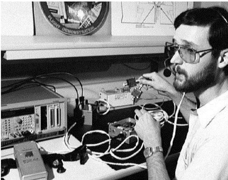
Joseph Prather is shown here with an infrared communications flight experiment (IRCFE) being readied for a flight on board the 1988 Space Shuttle Discovery STS-26 mission. The system uses light to communication in much the same way that radio waves are commonly used. [NASA/JSC news photo, released.]
