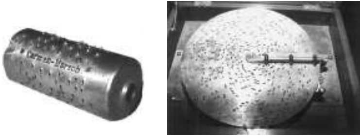
Coding systems allows sounds to be replayed. Left: Carmen-Marsch music cylinders from a table-top music box were like cartridges, interchangeable. The pegs would hit the sound mechanism as the cylinder rotated, producing the music. Right: A flat metal cylinder punched with holes to play a tune, housed in a phonograph-style cabinet, from the Bellingham Antique Radio Museum collection. [Classic Concepts photos ©1998, used with permission.]
