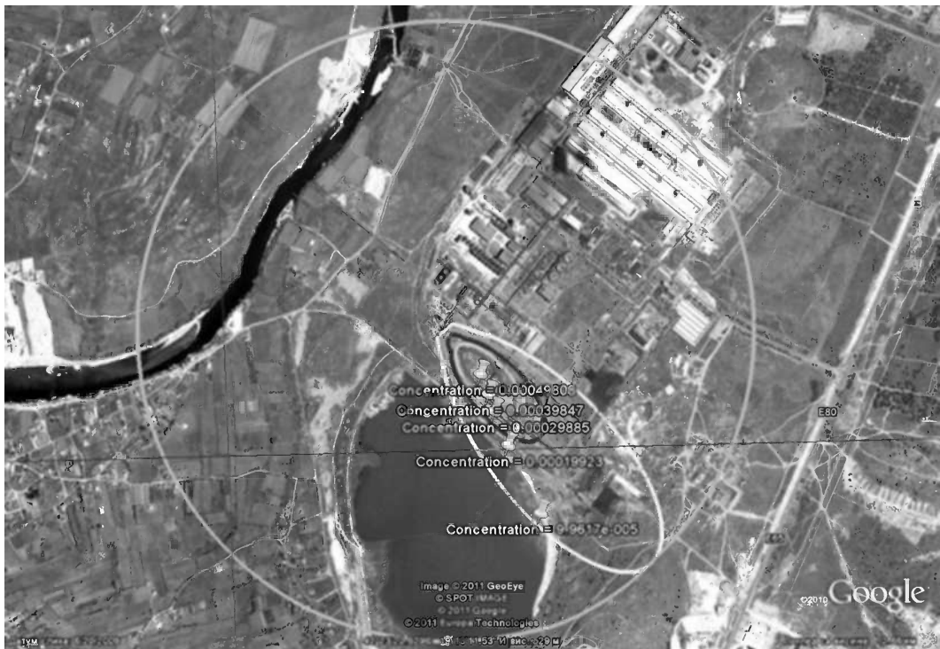
Figure 15.11 Levels of concern, case study of the Aluminium Plant Podgorica, using the GEPSUS program.
