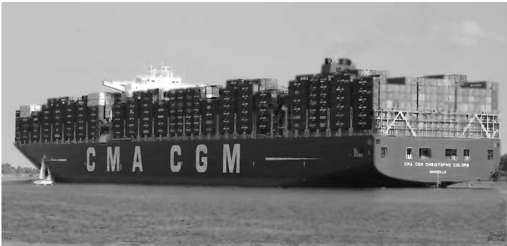
Figure 20.2 ULCS CMA CGM Christophe Colomb Carries 13,344 TEU. (Image Courtesy of H. Uet; Uet, H., CMA CGM Christophe Colomb 01.jpg, Wikimedia Commons, Available at http://commons.wikimedia.org/wiki/File:CMA_CGM_Christophe_Colomb_01.jpg , 2012.)
