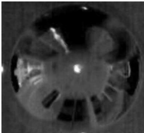
Figure 16.21 Thermal image captured through hyperbolic reflector.
