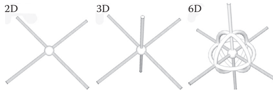
Figure 19.7 Examples of vector antenna. The 2D-vector antenna is composed by two orthogonal, colocated dipoles; the 3D-vector antenna is composed by three orthogonal, colocated dipoles; and the 6D-vector antenna is composed by three orthogonal, colocated dipoles and three orthogonal, colocated loops.
