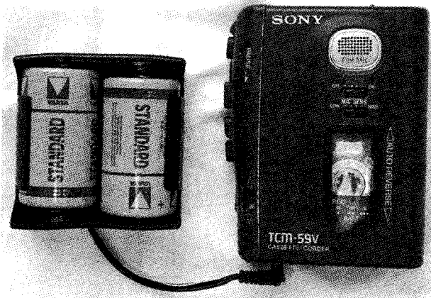
External power pack connected to tape recorder for longer recordings
