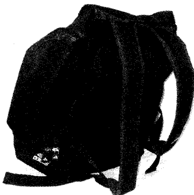
This rucksack has a pinhole lens in the shoulder strap. The recorder is concealed in the base
