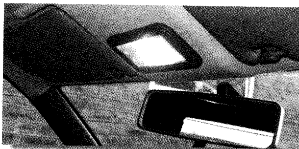
Disable interior lights if working at night
