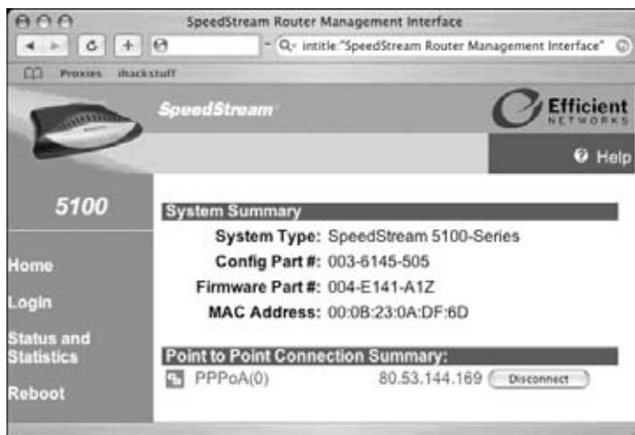
Figure 11.7 Open SpeedStream DSL Router Allows Remote Disconnects
