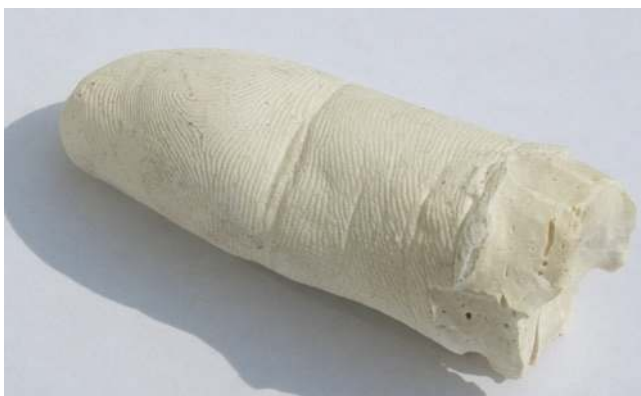
Fig. 6.21 Silicone cast of a finger. Note the friction ridge detail. First, a silicone mold was made, then the mold was used to produce the silicone finger
