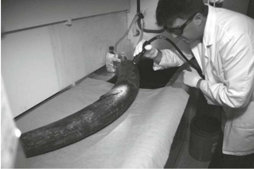
Fig. 21.6 Processing an intercepted shipment of elephant ivory tusks for latent prints using dyes and a monochromatic light source
