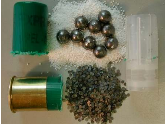
Fig. 9.12 Typical nine-pellet 00 buckshot load (shot shell was cut in half to remove the contents – clockwise from top, center pellets and buffer, shot cup, gunpowder, two halves of shot shell)
