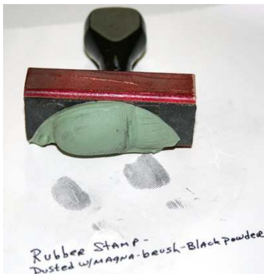
Fig. 6.21 Silicone cast of a finger. Note the friction ridge detail. First, a silicone mold was made, then the mold was used to produce the silicone finger
