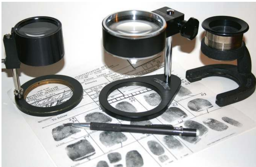
Fig. 6.9 Basic tools of the fingerprint examiner. Depicted here are three examples of adjustable low-power magnifying glasses and a tool called a ridge counter. The ridge counter aids the examiner in locating minutiae or identifying features that make up the friction ridge impression
