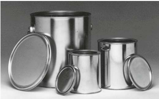
Fig. 5.7 Metal cans are used to collect arson samples
