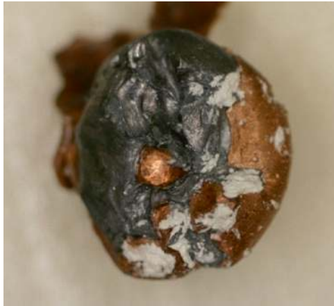
Fig. 9.11 Bullet with imbedded pulverized glass
