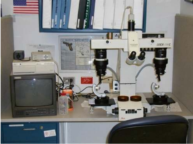
Fig. 9.14 Comparison microscope (image courtesy of James Gannalo, Det. NYPD ret.)
