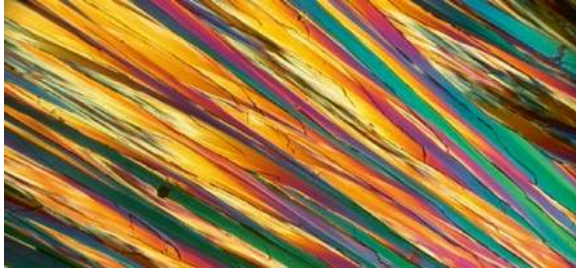
Fig. 5.14 Organic explosives using the polarized light microscope
