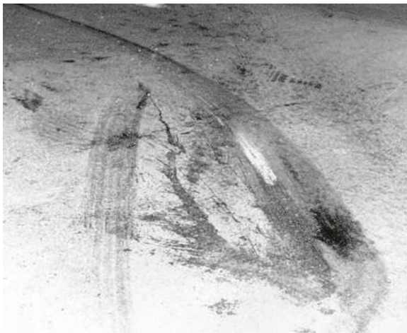
Fig. 20.1 Clearly visible point of impact (POI) on the roadway surface. Note the locked-wheel skid mark, the gouge markings, and the presence of fluid debris evidence
