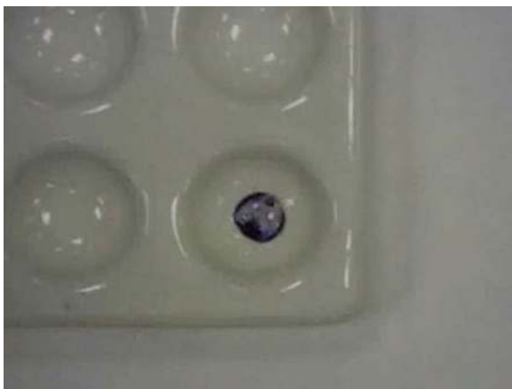
Fig. 5.9 The diphenylamine color test gives a dark blue color with both organic and inorganic nitrates as well as chlorates
