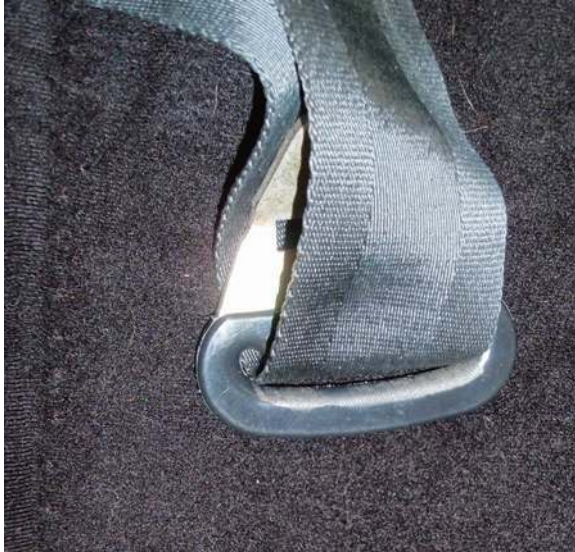
Fig. 20.5 Seat belt and D-ring removed from a vehicle following a serious crash. Note the clearly visible (striated) loading marks from the seat belt webbing on the D-ring. Loading marks are not always quite so well defined and readily apparent. Careful examination of the seat belt components, under magnification, should always be performed, if necessary
