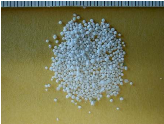
Fig. 9.13 Shot shell buffer (scale in mm)
