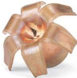
Fig. 9.10 Hollow-point bullet (expanded due to impact with a target)
