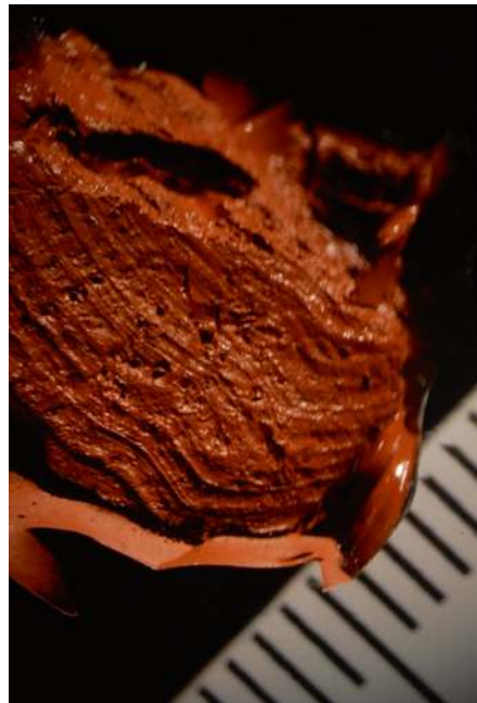
Fig. 19.25 Saw mark. Note the irregular, stepped striations in the cut surface
