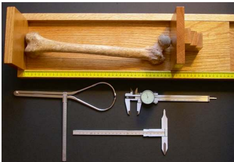
Fig. 19.16 The maximum length of the femur measured with an osteometric board. Below the osteometric board are spreading calipers (left) and two types of sliding calipers
