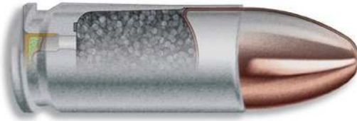
Fig. 9.9 Typical center fire cartridge (phantom view – image courtesy of RCBS Corporation)
