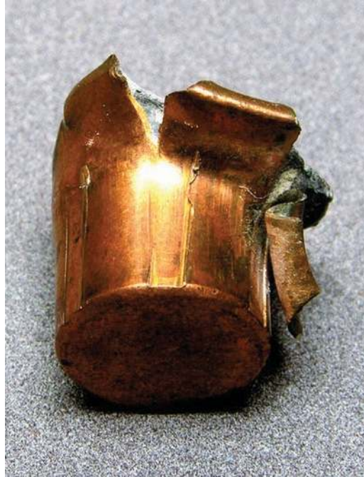
Figure 6.13 SEMIJACKET .45 Macro close-up of .45-caliber semijacket hollow point. Base view. (Courtesy of Detective Mark Czworniak, Chicago Police Department.)
