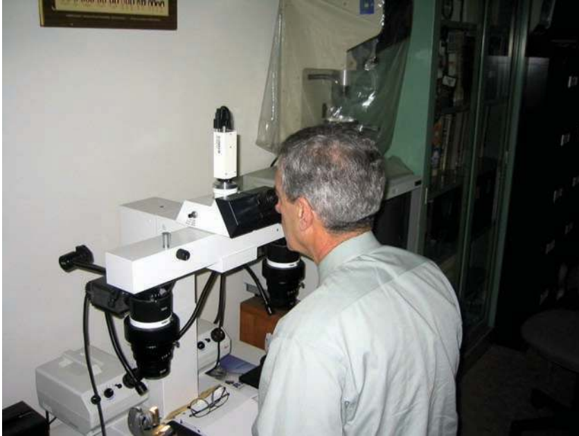
Figure 17.26 LEICA DMC COMPARISON MICROSCOPE. Detective Sergeant Frank Nicolosi is using this microscope, which consists of two optically paired microscopes connected to an optical bridge that allows the user to observe two objects simultaneously with the same degree of magnification. (Courtesy of Detective Sergeant Frank Nicolosi and Detective Sergeant Anthony Tota, Westchester County, New York, Police Department’s Ballistics Unit.)
