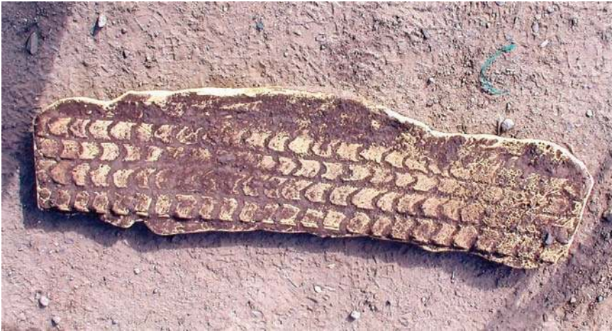
Figure 17.55 TIRE IMPRESSION. This photo depicts a 3-foot long cast of a tire impression using dental stone. (Courtesy of William J. Bodziak, supervisory special agent [retired], FBI Laboratory Division and author of Footwear Impression Evidence .)
