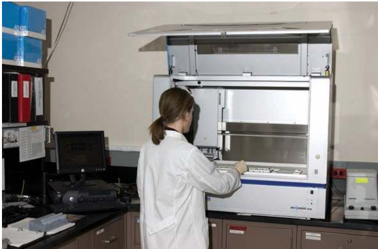
Figure 16.10 THE QIAGEN M48 BIROBOT. The Qiagen M48 BioRobot is designed to make the extraction of DNA samples less time consuming. The robot automatically transfers reagents and samples from tube to tube using magnetic beads to hold the DNA and allow its purification. (Courtesy of Fred Drummond, chief of Forensic Sciences, Westchester County, New York, Forensic Laboratory. Photographer: Keith Mancini.)
