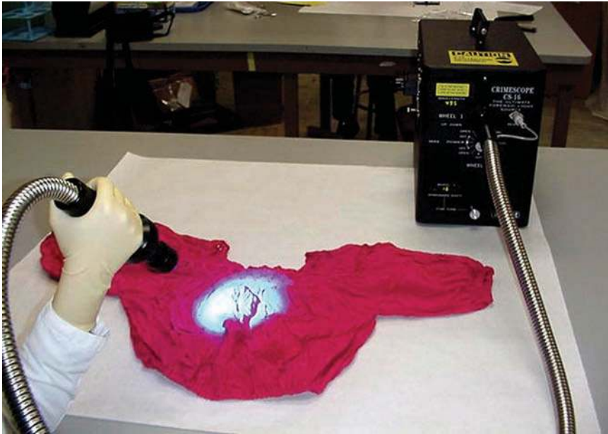
Figure 17.9 USE OF ALTERNATE LIGHT SOURCE. This photo illustrates the use of an alternate light source (ALS). The forensic scientist is examining clothing for body fluids not visible under normal lighting conditions. (Courtesy of Fred Drummond, chief of Forensic Sciences, Westchester County, New York, Forensic Laboratory. Photographer: Carlos Morales.)
