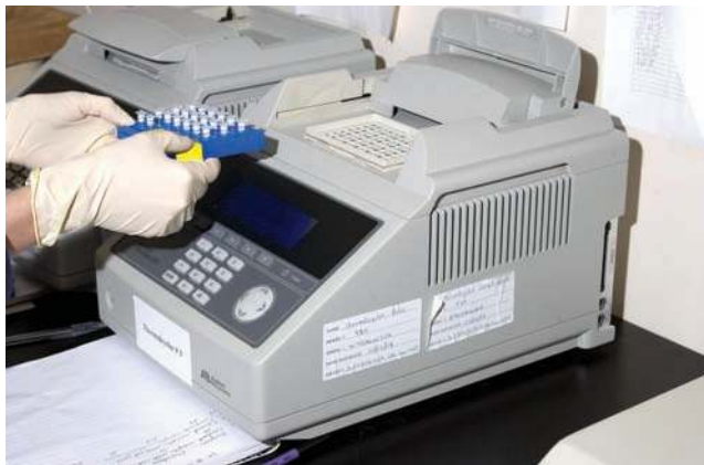
Figure 16.13 THERMAL CYCLER. The thermal cycler is used to carry out the polymerase chain reaction (PCR) for replication of forensic DNA samples. (Courtesy of Fred Drummond, chief of Forensic Sciences, Westchester County, New York, Forensic Laboratory. Photographer: Keith Mancini.)
