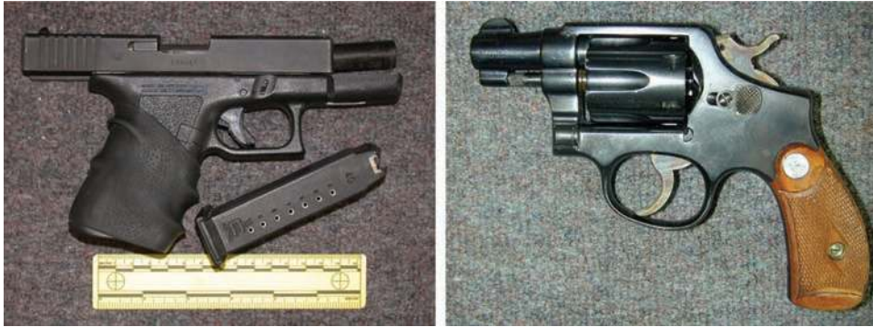
Figure 7.8 Two common types of handguns. On the left a semiautomatic pistol (with associated magazine); on the right a revolver.
