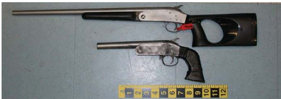
Figure 7.20 The weapon on top is an unmodified 410 shotgun; the lower weapon is a shortened version of the same model. The shorter barrel of the modified shotgun will change the characteristics of the shot patterns as compared to the unmodified firearm.
