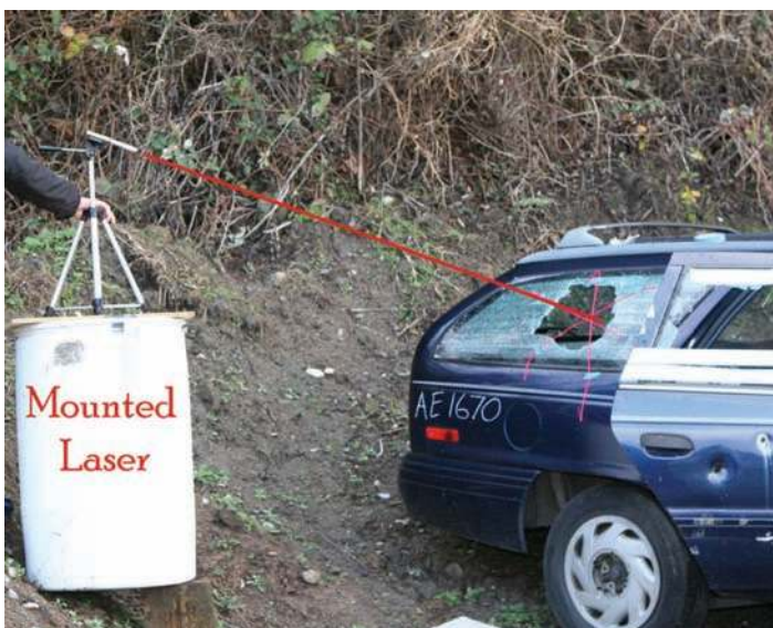
Figure 7.38 Lasers are often used in place of trajectory rods. The laser line is aligned with multiple defects and then photographed. The horizontal and vertical angle can be measured in the same fashion as when using a trajectory rod.
