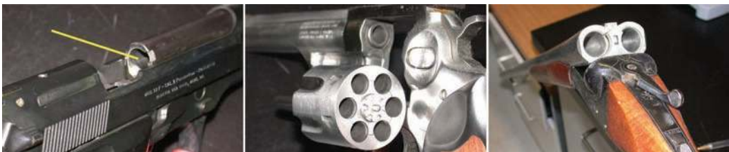
Figure 7.9 Chamber areas of a semiautomatic pistol, revolver, and side-by-side shotgun.
