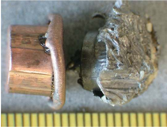
Figure 7.18 Shown is a fired bullet where the jacket separated from the core. These two components represent only one shot, so they should not be counted as two bullets. Notice the material trapped as trace evidence on each component.
