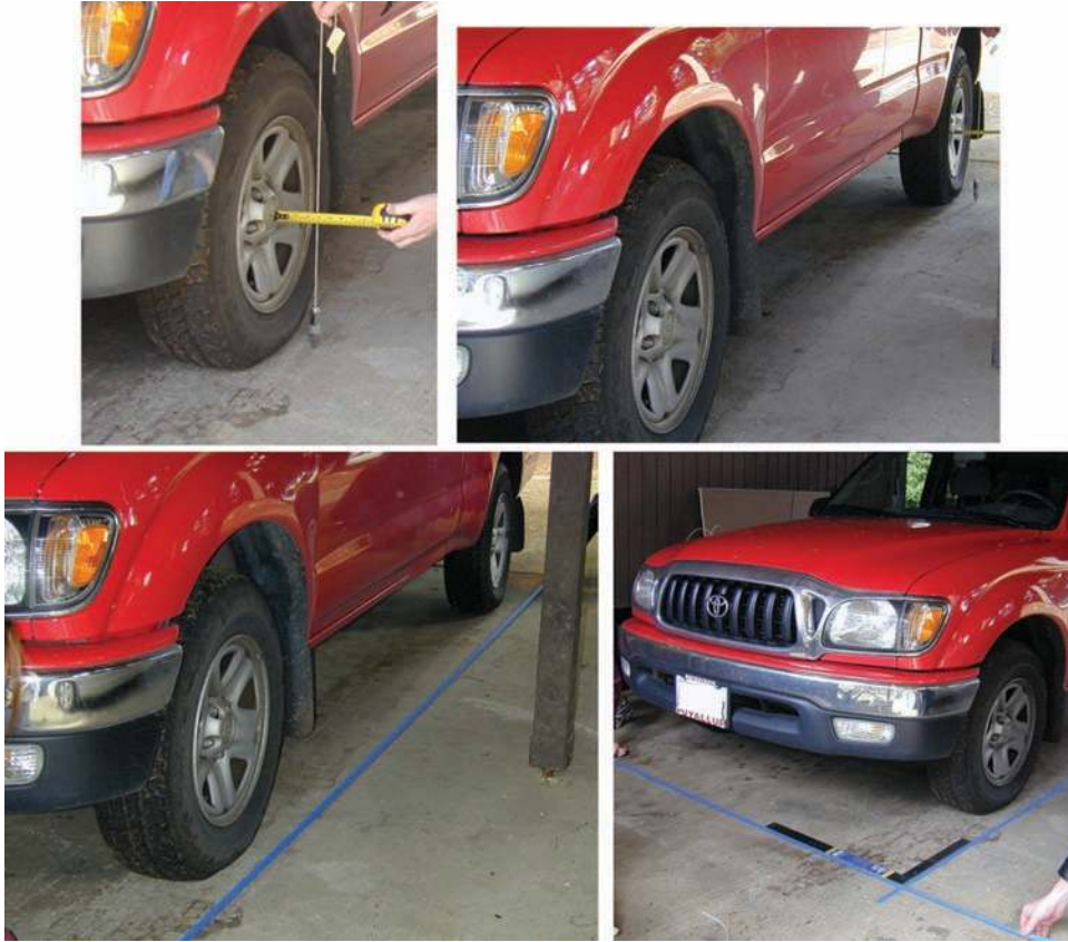
Figure 7.40 Providing external reference lines for vehicles is also known as “squaring a vehicle.” Mark an equidistant reference from two points on the side, connect the points, mark the front plane, and connect via a carpenter square.
