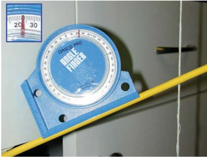
Figure 7.37 Vertical angle measurement reading the angle directly from an angle finder is pictured. The angle is downward at approximately 23 degrees (-23 degrees).
