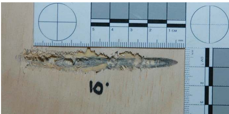
Figure 7.29 A ricochet from a .22 caliber bullet that originated from 10 degrees off the wooden surface. Direction of travel is from right to left and the elliptical black mark toward the right of the defect is a "lead-in" mark.
