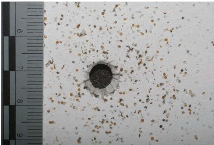
Figure 7.43 Shown is a pattern of gunpowder particles surrounding a bullet hole. This test shot was delivered onto paper from a .45 caliber pistol at 6 inches away. The multicolored disks are partially burned gun powder particles.
