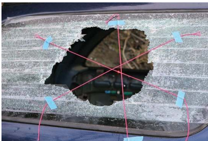
Figure 7.26 Even though the window has partially fallen in, the approximate area of initial perforation can be estimated by tracing the radial fractures back along their long axis.
