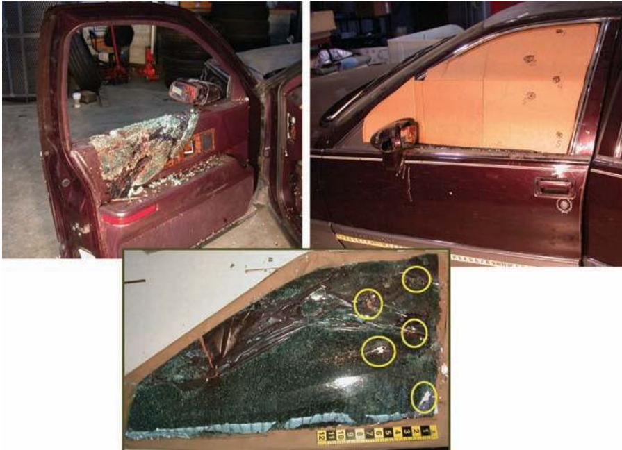
Figure 7.27 This tempered glass car window received multiple shots and the pane ultimately collapsed. The window tinting held the glass mostly together. It was recovered and, from it, the first shot was identified and a template of the bullet damage was applied to the reconstruction of the shooting scene.
