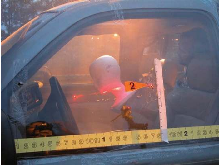
Figure 7.28 Another method of reconstructing glass and bullet defects. Using a scene photograph (before the pane collapsed) to identify the position of a bullet defect, this clear plastic template was created. It was then inserted into the vehicle and the laser aligned with the terminal defect. When considered in conjunction with a gunshot wound to the victim's chin, a general understanding of the victim's position is possible.
