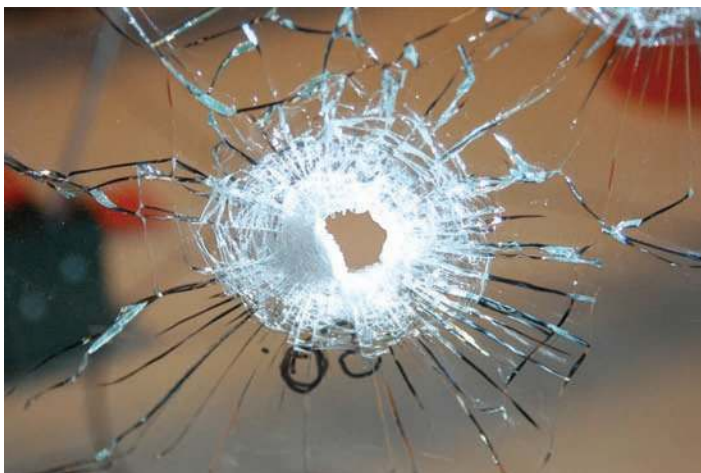
Figure 7.24 The view of the exit side of a bullet hole that went through laminated windshield glass.
