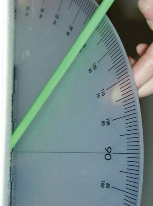
Figure 7.36 Vertical angle measurement recorded using a protractor. Reading the protractor on scene identified the angle as downward at approximately 40 degrees relative to level (–40 degrees). However, because the photograph was not taken properly (it is not taken parallel to the rod), actually measuring the angle from the photo will result in the incorrect angle of –55 degrees—a significant error.
