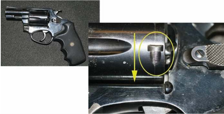
Figure 7.12 The stops on a cylinder can indicate which direction the cylinder is designed to rotate. Here, the lead into the stop is on the lower side of the notch identifying that this cylinder rotates to the left (from the shooter’s perspective).
