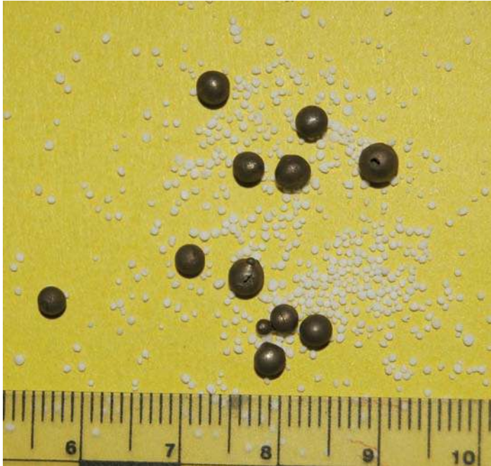
Figure 7.23 Shot pellets among buffer component, which is added to reduce the interaction of the pellets when fired.
