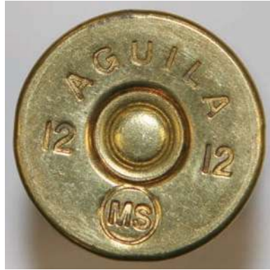
Figure 7.5 The head of the cartridge—the headstamp identifies the manufacturer: Aguila; the caliber: 12 (Gauge); and the symbol: MS for minishell.
