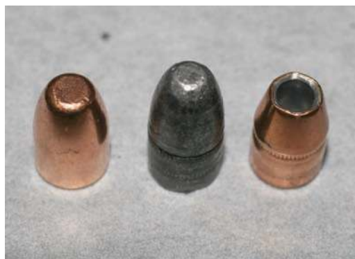
Figure 7.4 Three different projectile designs—a .38 special full metal jacket (FMJ), a .38 Special lead round nose (PbRN), and a .38 Special jacketed hollow point (JHP).
