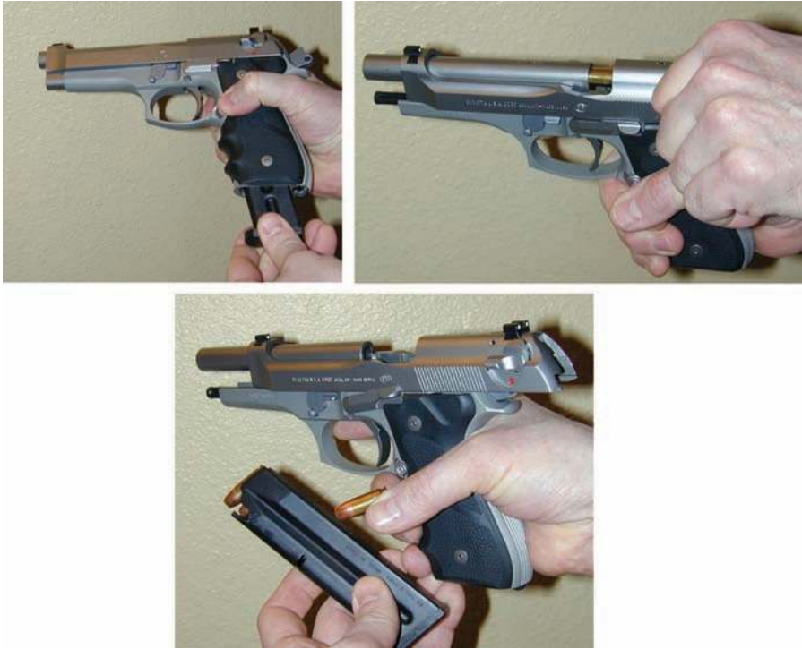
Figure 7.14 The normal sequence to unload a semiautomatic pistol: drop the magazine; expose and clear the chamber; package all items.
