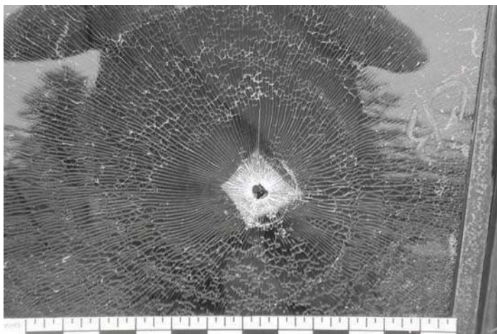
Figure 7.25 Fractures radiating out from the impact site on a shot fired through tempered glass. The long narrow fractures will point back to the position of initial impact.
