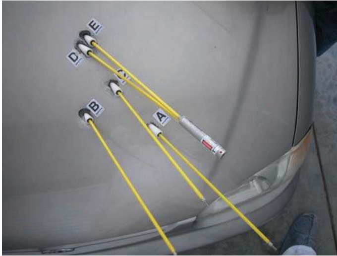
Figure 7.42 A demonstrative photo of multiple trajectory rods. Because of the perspective this photo was taken at, the angles in the photo cannot be used to calculate the true angles recorded at the scene. It simply demonstrates that the bullets were striking the vehicle on the right from a position forward of the driver's door.
