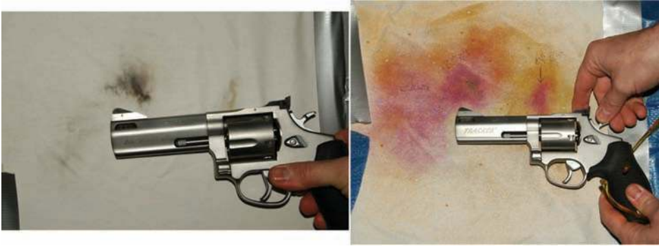
Figure 7.44 A revolver fired adjacent to the wall left residue defining the distance between the cylinder gap and muzzle. At right, the sodium rhodizonate reagent was used to develop the vaporous lead in the pattern.
