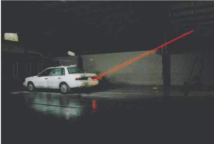
Figure 7.39 This laser trajectory was photographed using a bulb setting and paint with light technique.
