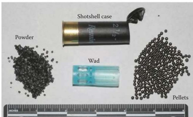
Figure 7.6 A schematic and disassembled shotshell.
