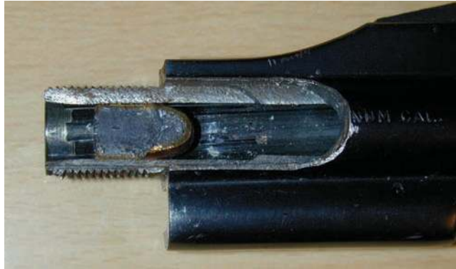
Figure 7.10 A cut-away firearm barrel showing a lodged bullet and the barrel lands and grooves.
