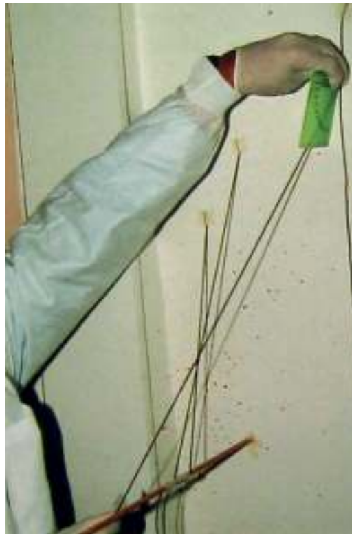
Figure 2.14 Bloodstain pattern analysis using 'stringing'. (Reproduced from James, S.H. et al. , (2005) Principles of Bloodstain Pattern Analysis , Copyright © 2005, Taylor & Francis.)
