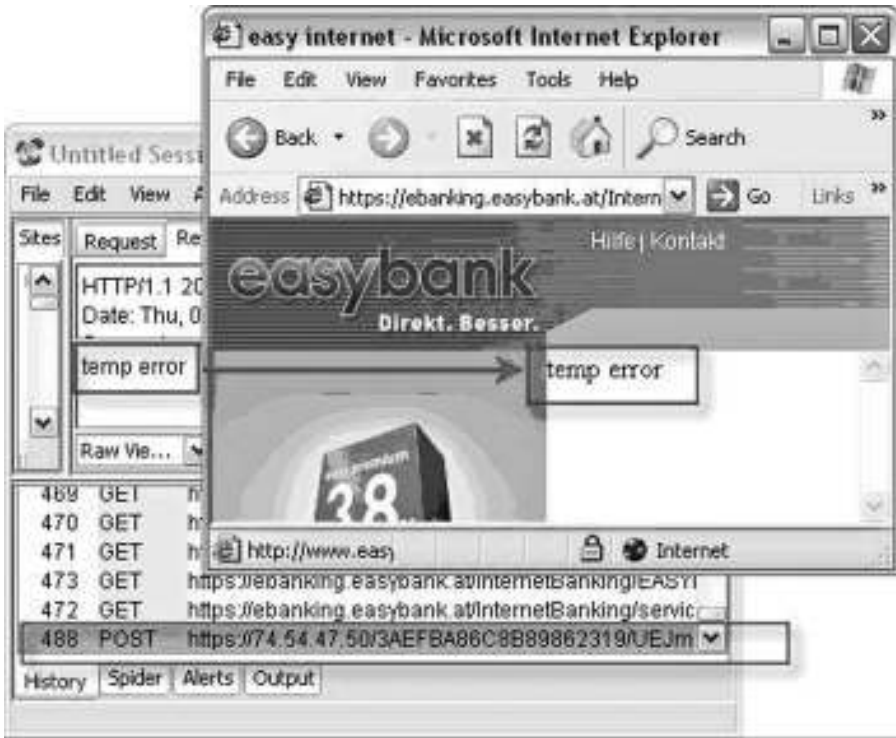
Figure 10.19 MaOS frequently displays “temp error,” a visual cue of infection.
