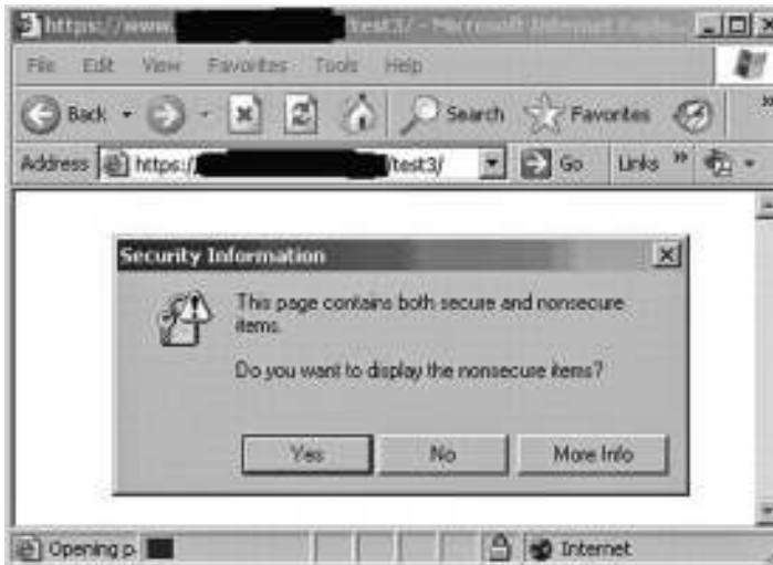
Figure 8.4 The warning that is displayed when an HTTPS site loads an HTTP IFrame.
