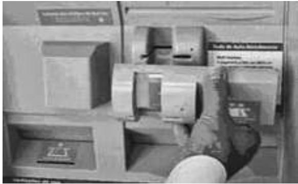
Figure 4.17 A skimmer, or “chupacabra,” in Portuguese, installed on an ATM of a prominent Brazilian bank.
