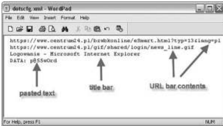
Figure 13.16 SilentBanker logs intercepted “paste” text to dotscfg.xml.
