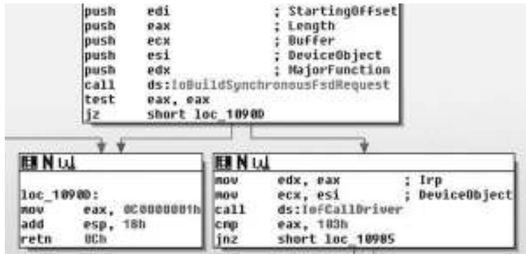
Figure 10.10 Direct disk access circumvents security monitors.
