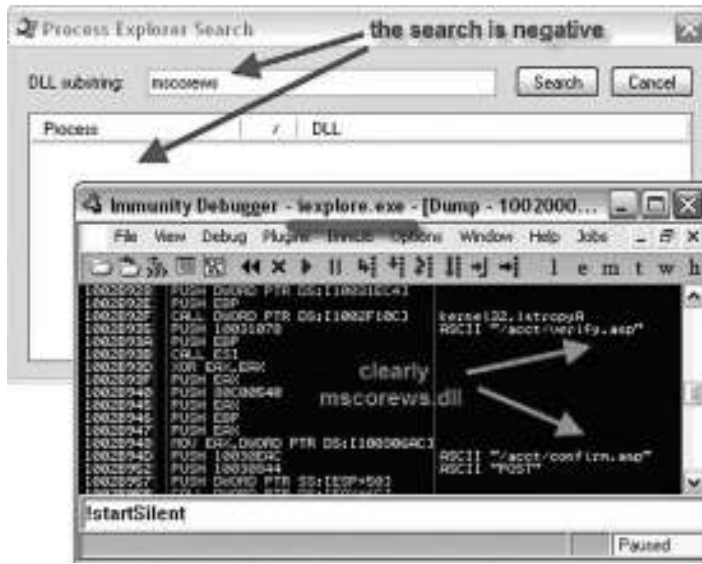
Figure 13.2 SilentBanker code inside Internet Explorer is undetected by Process Explorer.
