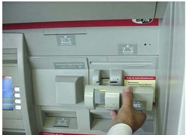
Figure 7.6 ATM Skimmer Device.
