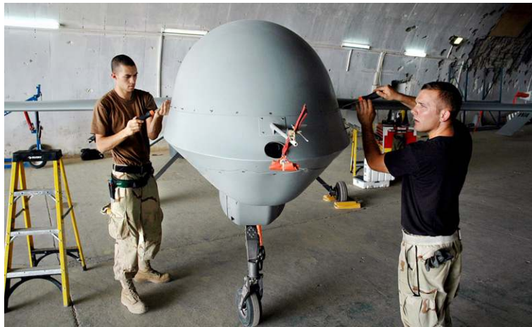
FIGURE 10.2 Airmen attach the radome to an MQ-1 Predator unmanned aerial vehicle at Balad Air Base, Iraq, in 2005. Photograph from www.defense.gov , taken by Maj. Robert Couse-Baker.
