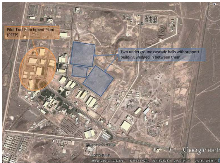
FIGURE 13.1 GoogleEarth image of Natanz' Fuel Enrichment Plant (FEP) and the Pilot Fuel Enrichment Plant (PFEP). Image copyright 2012, Google.
