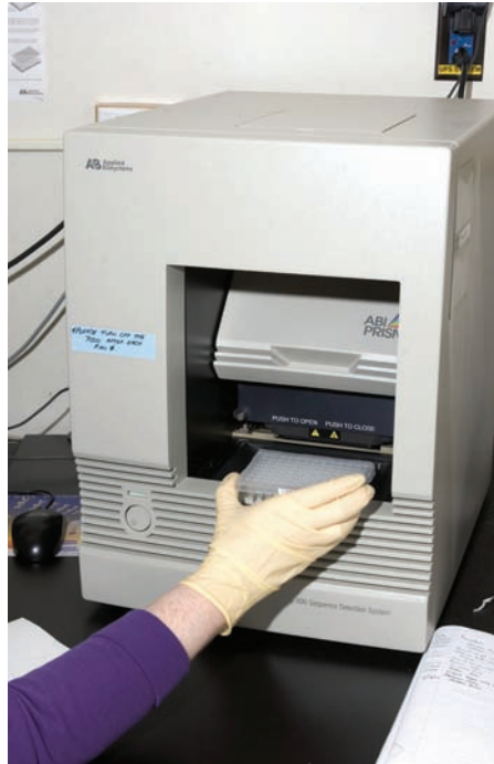
Figure 16.12 REAL TIME PCR. “Real time PCR” is a new technique used to determine the quantity of DNA present in a sample relative to a set of standards. It works by amplifying the DNA in each sample with fluorescent primers. The change of fluorescence is recorded by camera and analyzed by a computer. The calculated value is used to determine the amount of amplifiable DNA present in a sample. (Courtesy of Fred Drummond, chief of Forensic Sciences, Westchester County, New York, Forensic Laboratory. Photographer: Keith Mancini.)
