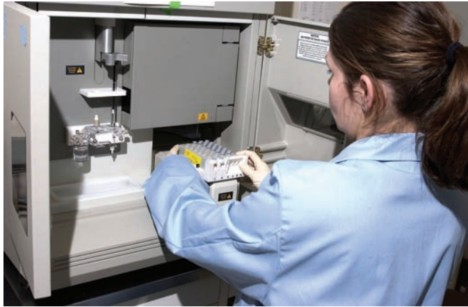
Figure 16.17 CAPILLARY ELECTROPHORESIS UNIT. Forensic analyst Jennifer Reilly places samples in the ABI Pism 310 capillary electrophoresis (CE) unit. This instrument will analyze fragments of DNA to obtain a genetic profile. (Courtesy of Fred Drummond, chief of Forensic Sciences, Westchester County, New York, Forensic Laboratory. Photographer: Keith Mancini.)
