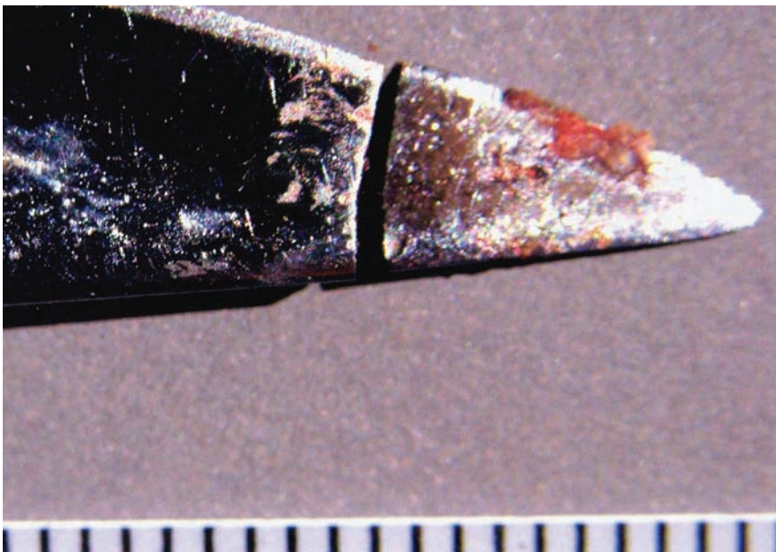
Figure 18.28 FRACTURE MATCH. This photo shows the "fracture match" of the tip of the blade removed from the chest of the victim by the medical examiner to the murder weapon recovered by the police. The only undisputed and conclusive method of identifying a sharp-bladed instrument to the actual stab wound is to recover a piece of the weapon within the wound structure and match it to the murder weapon. (Courtesy of Detective Mark Czwozniak, Chicago Police Department.)
