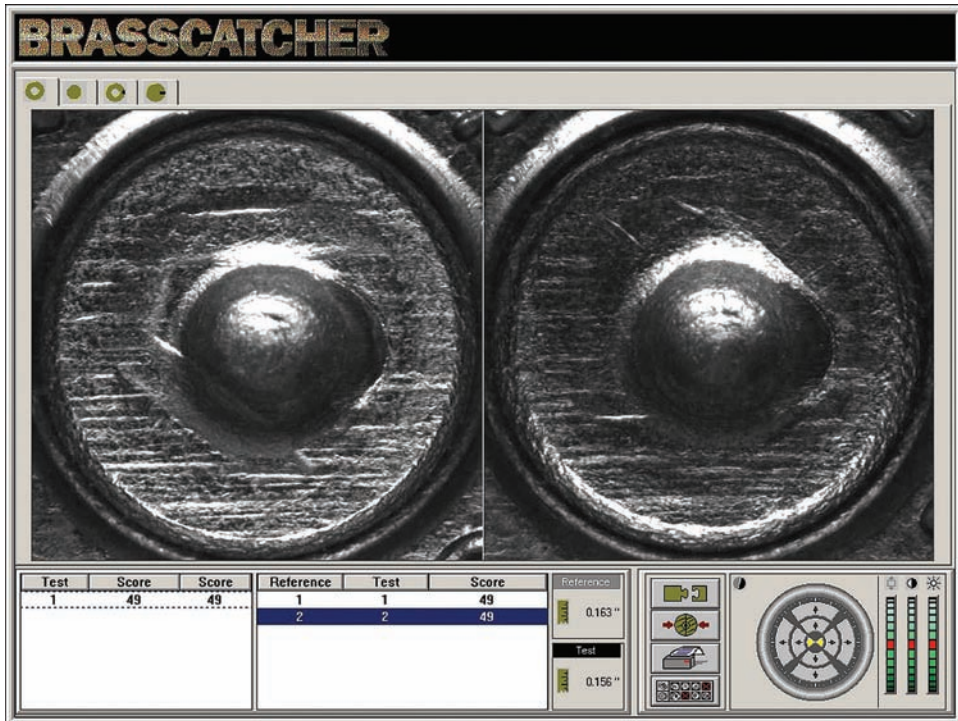
Figure 17.31 IBIS BRASSCATCHER FOR CARTRIDGE CASE. Screen depicting side-by-side comparison of cartridge cases. (Courtesy of Forensic Technology, Inc., 888/984-4247, www.forensictechnologyinc.com .)
