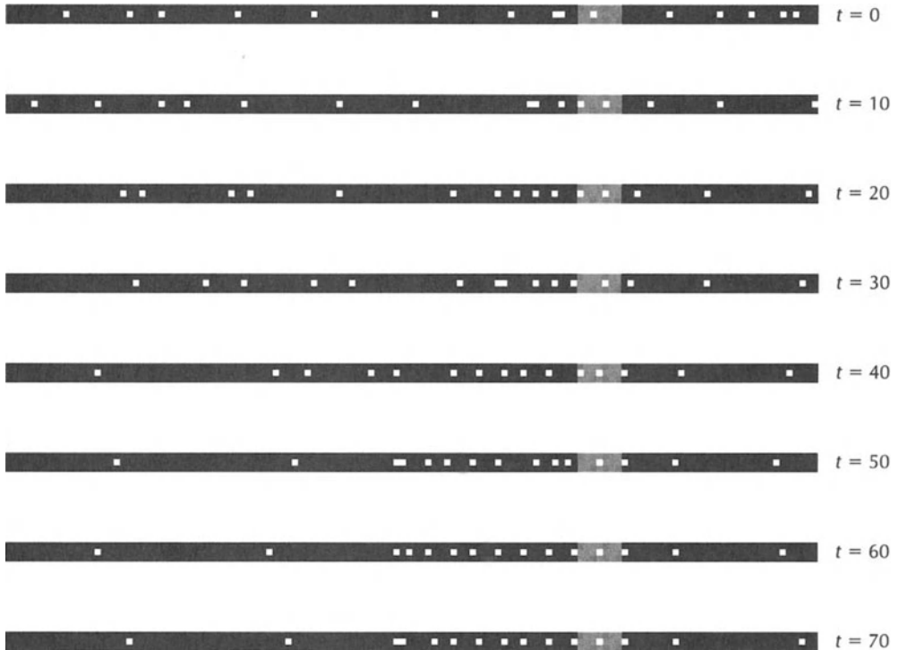
FIGURE 5.2 Traffic Jams Caused by Radar Trap (shaded area). (Cars move left to right.)
