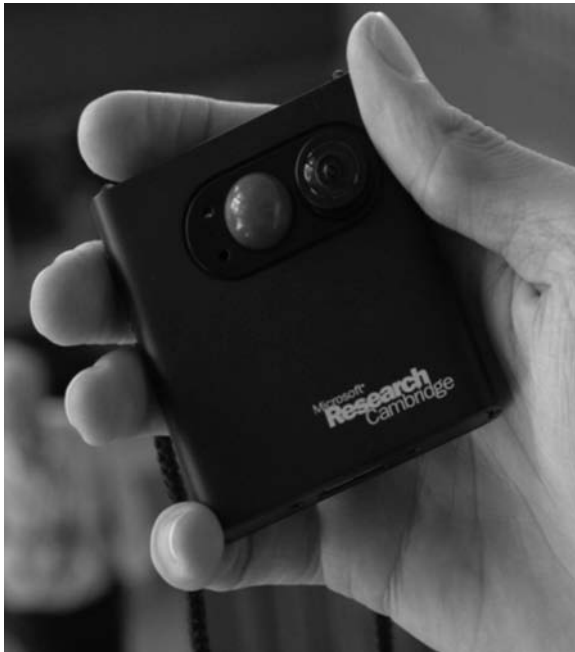
Figure 2.7 Microsoft's SenseCam (wearable digital camera) and some sample shots taken by camera as a function of sensor change elicited by the wearer's movement or background change.
