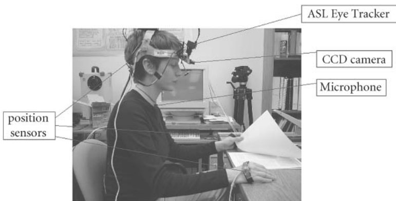
FIGURE 10.4. The computational model shares multisensory information like a human language learner. This allows the association of coincident signals in different modalities.
