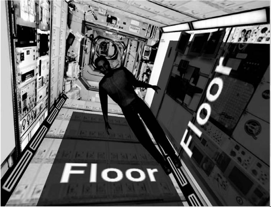
Figure 13-9. VRI in the ISS US Laboratory module. The equipment and labeling on the true floor and ceiling are oriented 90 degrees counterclockwise from those on the true walls and floor. The square cross section of the module means the major physical axes of symmetry are also 90 degrees apart. When a crewmember floats in this body orientation, which surface is perceived as a floor depends on visual attention. VRIs due to such ambiguities can only be prevented by attending to learned landmarks.
