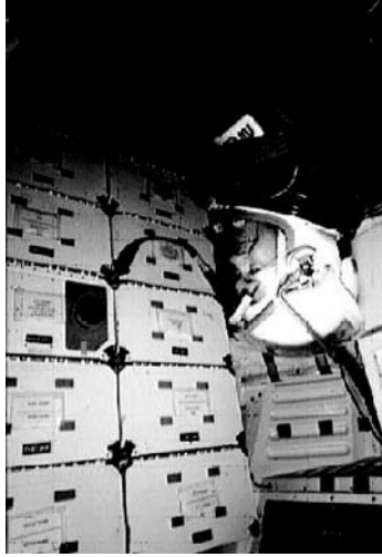
Figure 13-2. Persistent 0-G Inversion Illusion – both self and vehicle seem upside down relative to an unseen external gravitational reference frame. The illusion is often reported in the Shuttle mid-deck, where walls of rectangular stowage lockers make up and down ambiguous (NASA photo)
