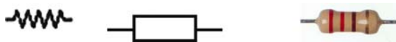
Fig. 5.123. Representatives of the resistor as a electronic symbol and a real-world object
