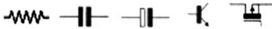
Fig. 4.4. The category of electronic symbols: a resistor, a capacitor, a capacitor electrolytic, a bipolar transistor, a field-effect transistor
