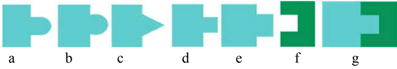
Fig. 5.112. Assembling two parts: (d–e) objects that are representatives of the compatible components, (a–c) objects that are representatives of the noncompatible components, (e) a basic component, (g) the whole object
