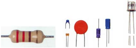
Fig. 4.43. The category of electronic elements the resistor, capacitor, capacitor electrolytic, bipolar transistor, field-effect transistor
