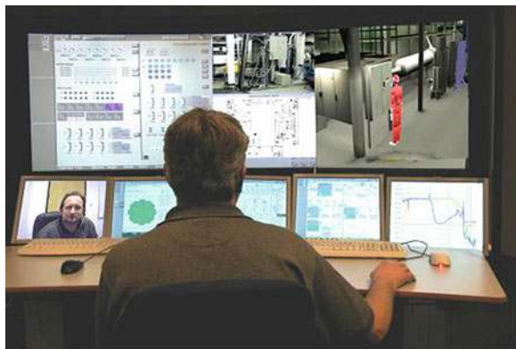
Fig. 2.19 The “cockpit control room” implemented in HAMMLAB for the Extended Teamwork experiment
