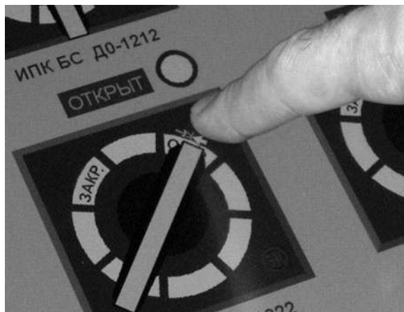
Fig. 8.9 Conventional instrumentation represented using a flat touch screen at the Leningrad Nuclear Power Plant Validation Facility
