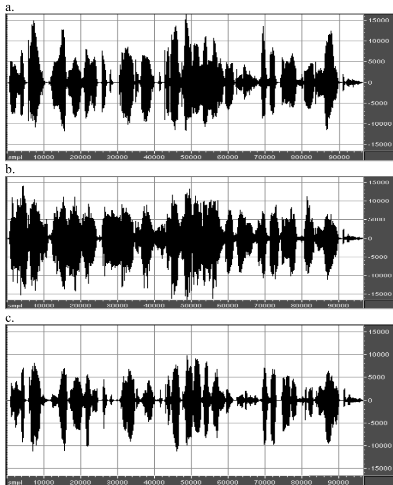
Fig. 5.41. Filtration of two sentences (time domain representation); original signal before processing (a); signal mixture – original signal + disturbing signal from 45^\circ (b); result of NN-based filtration (c)
