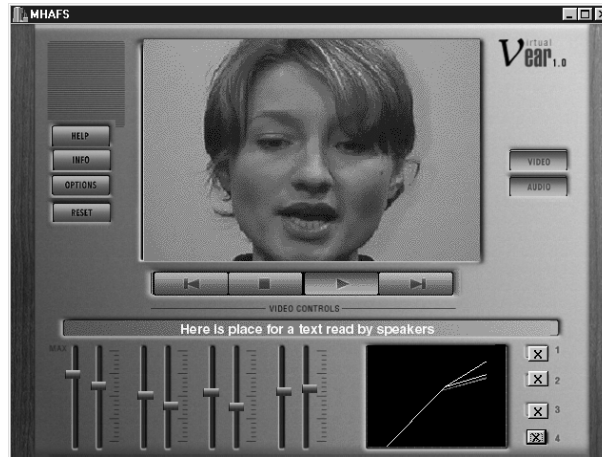
Fig. 5.23. User interface design. In the lower part of the computer screen sliders are seen which make it possible to change the shape of compression curves within the interest region
