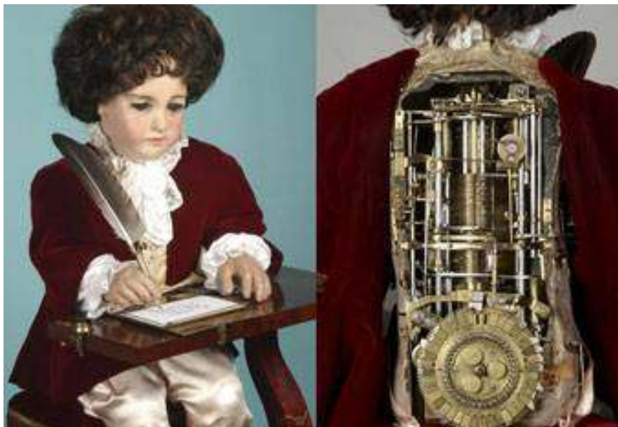
Fig. 2 The Jaquet-Droz brothers' automata (built at the end of the XVIII century) are an example of the level of complexity of behavior and realistic appearance that a purely mechanical automata, based on gears, Geneva wheels, cams and belts can reach. Three of these automata (the writer, the drawer and the player) are conserved in the Neuchâtel Museum of Art and History. The writer, the most complex can be 'programmed' to write any given text with a maximum of 40 letters long. He inks his goose feather at regular times. His gaze follows the text while writing and move the head accordingly when he inks the pen. Similar examples of the same age are the Japanese Karakuri dolls (Courtesy: Neuchâtel Museum of Art and History).
