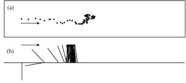
FIG. 2. Illustrative examples of causal entropic forcing. (a) A particle in a box is forced toward the center of its box. (b) A cart and pole system in which only the cart is forced successfully swings up and stabilizes an initially downward-hanging pole. (See also Supplemental Material, Movies 1 and 2 [13], respectively.)
