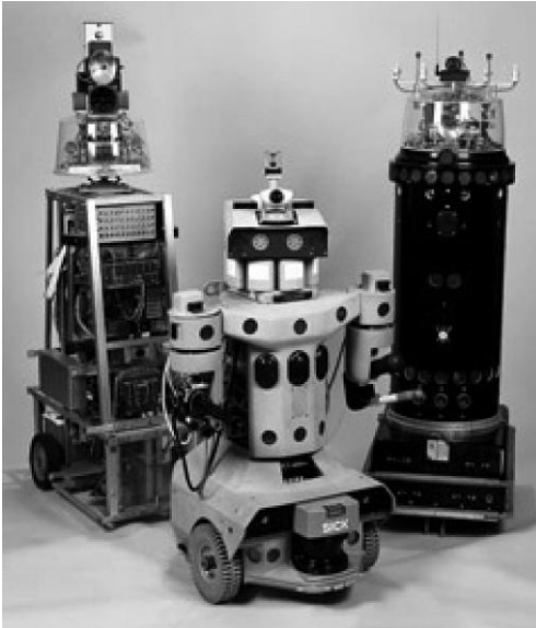
Left: The earliest Robart surveillance robot was only capable of sensing an intruder. Later versions added assessment and autonomous decision-making capabilities. Right: The Robart III's Vision Computer is housed in the head. It takes live video feeds from the robot's various cameras and converts them to digital images for storage and later processing and analysis. The robot also includes ladar (laser radar) and near-infrared sensors. [News photos courtesy of U.S. Navy SPAWARS, released.]
