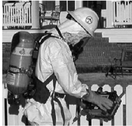
Left: Sandia National Laboratories maintains a state-of-the-art chemical and radiation-detection laboratory in California designed for researching chemicals, sensors, and detectors. Right: In 2008, prototype handheld chemical detectors were tested for emergency response suitability. Chemical suits protect first responders until it is known whether any toxins are in the area. [News photos courtesy of Sandia National Laboratories and the Department of Homeland Security, released 2008.]
