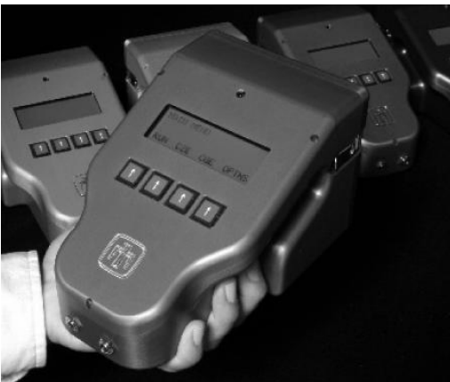
The portable bio-detection MicroChemLab developed by Sandia National Laboratories was found capable of detecting and analyzing toxic agents in laboratory tests, and was field-tested in the fall of 2003. The gas-phase device was initially developed for chemical warfare detection and emergency response, but also has applications for ecological monitoring and industrial process control. [News photos courtesy of Sandia National Laboratories, 2003 and 2011, released.]
