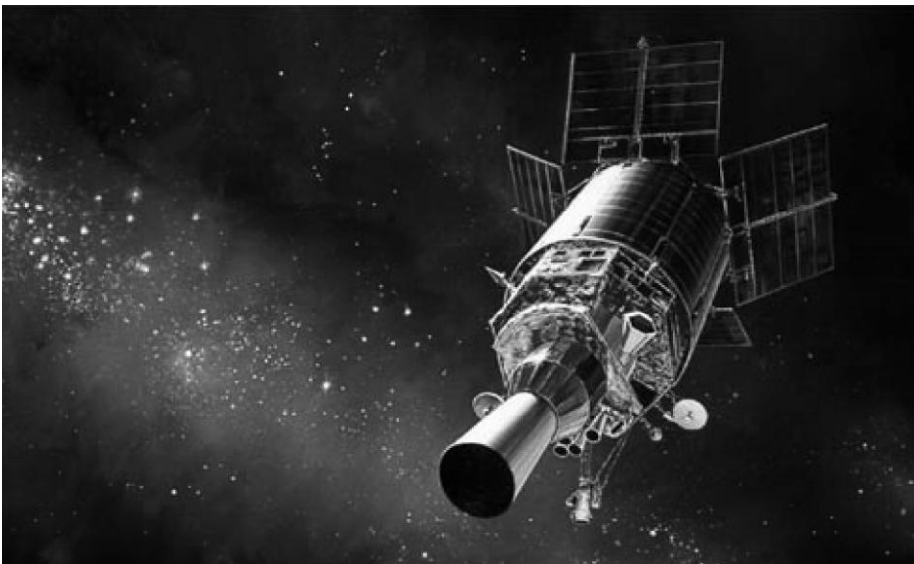
Geosynchronous surveillance satellites in the Defense Support Program provide early warnings by using thousands of infrared sensors to sense signs of heat emissions from explosions, missile launches, and nuclear detonations. If events are detected, reports are relayed to the North American Aerospace Defense Command and other strategic commands. The system has been in place since the 1970s and has gone through a number of upgrades to improve the number and quality of the sensors. [News photo courtesy of the U.S. Air Force, 2010, released.]
