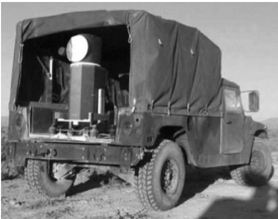
The JBSDS is a transportable biological agent detector for detecting biological agents at a distance. [News photo courtesy of the DoD, released.]
