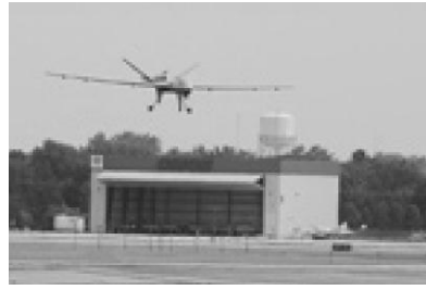
Left: The Predator B UAV is remotely controlled via C-band radio signals for line-of-sight and via Ku-band radio signals relayed through orbiting satellites for longer distances. It can stay aloft up to 20 operational hours and fly at altitudes up to 50,000 feet. Right, a CBP Predator B comes in for a landing at the Oshkosh airport in Wisconsin, representing a milestone UAV landing in a civilian airport. [News photos courtesy of CBP, 2010, released.]
