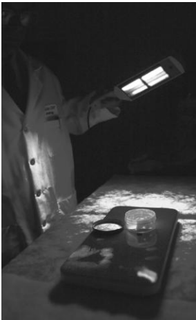
A Customs and Border Protection (CBP) lab worker holds up a black light —a light that emits frequencies that stimulate ultraviolet-sensitive materials like special inks and powders to glow (fluoresce). Ultraviolet lights are used for many forensic purposes by CBP and police departments to check for marked articles, signs of tampering, or incriminating traces of powder or gel that a thief might have on fingers or clothes. [CBP photo by James Tourtellote, 2006, released.]
