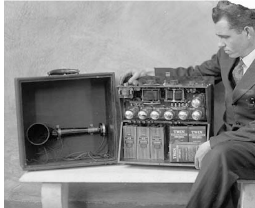
Left: Vacuum tubes were constructed in a great variety of shapes and sizes for different purposes until transistors and microelectronics made them obsolete (except for specialized applications). Right: Inventor Brent Daniel displays a historic portable super-heterodyne radio-wave receiving unit. Seven vacuum tubes can be seen in the cabinet. Inventions like this eventually led to military field radios and consumer portable radios. [Left: Vacuum tubes in the American Radio Museum courtesy of Classic Concepts, © 1997. Right: Harris & Ewing photo courtesy of the Library of Congress, public domain.]
