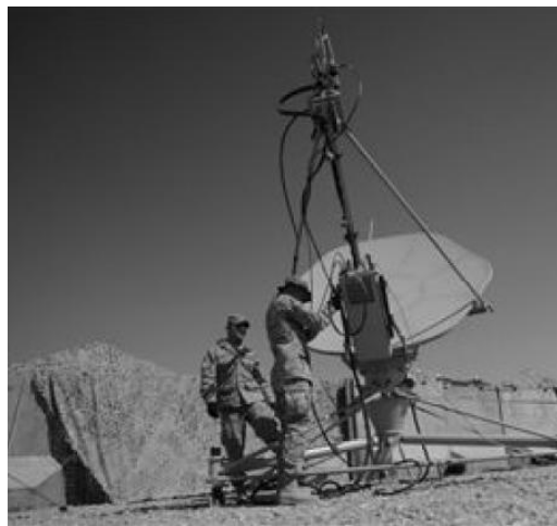
Left: U.S. Air Force crew adjust a microwave communications antenna atop a communications tower to provide wireless network access. Right: This transceiving dish was installed in Kandahar, Afghanistan, to provide wireless in-the-field telephone and Internet communications via orbiting satellites. [News photo by Staff Sgt. Mike Meares and Sgt. James Harper courtesy of the U.S. Air Force, 2011 and 2009, released.]
