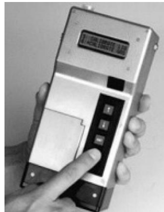
The portable bio-detection MicroChemLab developed by Sandia National Laboratories was found capable of detecting and analyzing toxic agents in laboratory tests, and was field-tested in the fall of 2003. The gas-phase device was initially developed for chemical warfare detection and emergency response, but also has applications for ecological monitoring and industrial process control. [News photos courtesy of Sandia National Laboratories, 2003 and 2011, released.]
