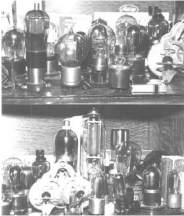
Left: Vacuum tubes were constructed in a great variety of shapes and sizes for different purposes until transistors and microelectronics made them obsolete (except for specialized applications). Right: Inventor Brent Daniel displays a historic portable super-heterodyne radio-wave receiving unit. Seven vacuum tubes can be seen in the cabinet. Inventions like this eventually led to military field radios and consumer portable radios. [Left: Vacuum tubes in the American Radio Museum courtesy of Classic Concepts, © 1997. Right: Harris & Ewing photo courtesy of the Library of Congress, public domain.]
