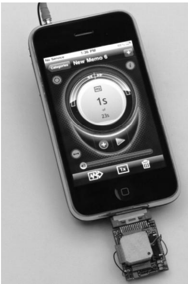
Jing Li, a scientist at NASA/Ames has developed a compact electronic chemical sensor (left) that can be interfaced with a cellphone docking station (right) to detect small amounts of chlorine gas, methane, and ammonia. The chip includes 16 nanosensors and can relay the information via the cellphone to another phone or computer. A newer version of the chip includes 16 nanosensors per side, for a total of 64 nanosensors. [NASA/Ames news photos by Dominic Hart, 2009, released.]
