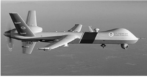
Left: The Predator B UAV is remotely controlled via C-band radio signals for line-of-sight and via Ku-band radio signals relayed through orbiting satellites for longer distances. It can stay aloft up to 20 operational hours and fly at altitudes up to 50,000 feet. Right, a CBP Predator B comes in for a landing at the Oshkosh airport in Wisconsin, representing a milestone UAV landing in a civilian airport. [News photos courtesy of CBP, 2010, released.]
