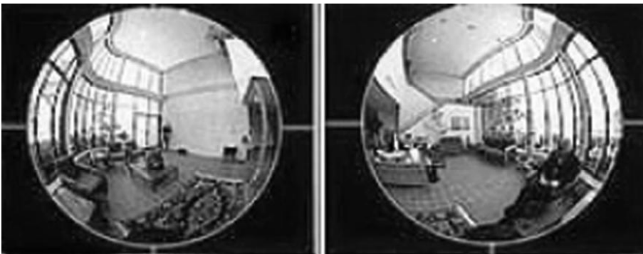
Fisheye lenses (about 8 to 10 mm) and wide-angle lenses give a broader field of view than typical lenses in the 50 to 200 mm range, but they also introduce distortion that increases toward the periphery. This may be an acceptable compromise for surveillance cameras but may create problems for other applications such as scientific imaging or scanning. Image processing algorithms and special lens arrays have been developed to provide larger imaging surface with less distortion. [Image courtesy of NASA, released.]
