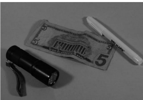
Articles can be marked for security and ownership identification with ultraviolet powder, paste, or ink (left) and the marks revealed later with a UV flashlight (right). This is helpful for marking valuables and can also be used for gate re-entry at amusement parks and temporary events, in the form of a hand- or card-stamp. People selling goods online often use UV to mark products to verify that a returned item is the original and not a substitute. In low-light conditions, a UV light reveals the otherwise invisible mark. [Photos copyright © 2012 Classic Concepts, used with permission.]
