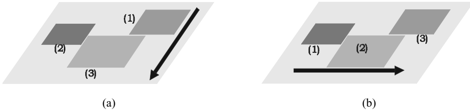
Figure 15.2 Geometrical control of the child-pad-activation order. (a) VerticalUpdatePad sends “update” messages to its child pads in either the ascending or descending order of their top-edge y coordinate. (b) HorizontalUpdatePad sends “update” messages to its child pads in either the ascending or descending order of their left-edge x coordinate.
