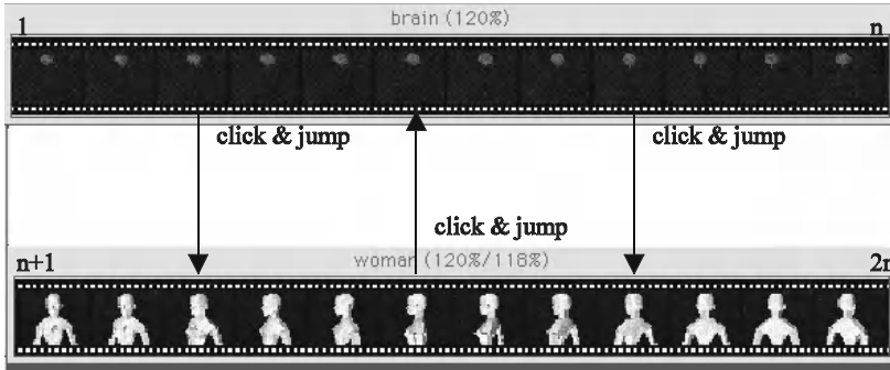
Figure 13.19 The example application of the frame jump function f(i) = i + n \text{ mod } 2n .
