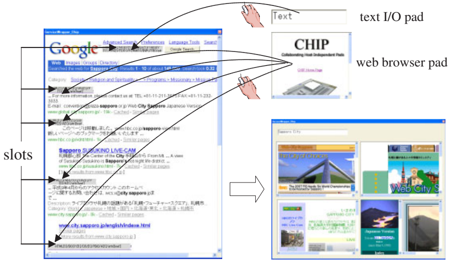
Figure 1.6 You can easily wrap the Google Web page to define a portal that shows the first four candidate Web pages for arbitrarily given keywords.
