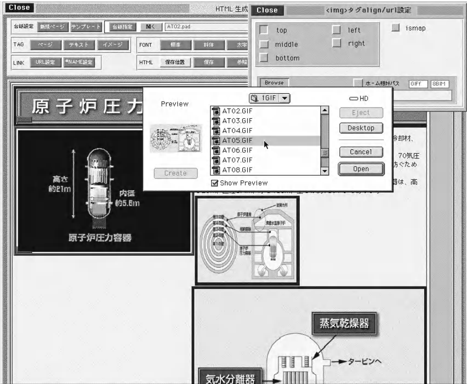
Figure 17.15 If you want to insert an image, you can first paste an image pad at a desired location, resize it, and then open its associated file selector to select an image file.
