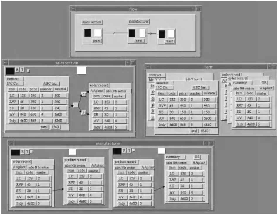
Figure 14.13 A display screen copy of an example form-flow system. The top middle composite pad defines a form flow using meta-pads.
