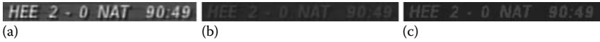
Figure 4.18 Original image (a), the result of general contrast reduction method (b), and the result of the proposed method (c) with C_1 = 1 , C_2 = 0 , and C_3 = 1 and I_{\max}^{\text{new}} = 50 .
