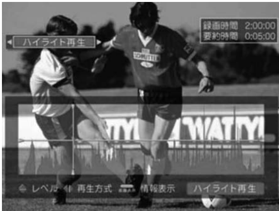
Figure 18.4 Video browsing enhanced personal video recorder. (From Divakaran, A. and Otsuka, I., A video-browsing-enhanced personal video recorder, in: 14th International Conference on Image Analysis and Processing Workshops (ICIAPW 2007) , Modena, Italy, pp. 137–142, 2007. © 2007 IEEE. With permission.)
