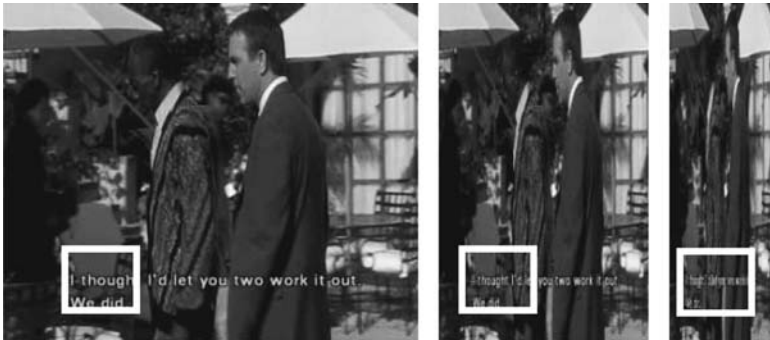
Figure 4.4 The proposed height-preserving multiresolution approach uses the same number of lines for the same window size (shown in white; window is larger than 11 \times 11 for better visualization of the concept). (From Ekin, A., Local information based overlaid text detection by classifier fusion, in Proceedings of the IEEE ICASSP , Toulouse, France, 2006. With permission. Copyright 2006 IEEE.)
