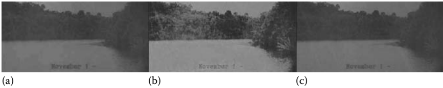
Figure 4.8 An image where text is most distinguishable in the color channel (original—(a), histogram equalized for display—(b)), but it has very low contrast in the luminance channel (c).
