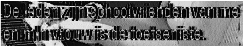
Figure 4.14 The artifacts caused by high peaking and LTI settings include thicker dark background and ghost effect in text regions.
