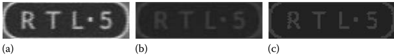
Figure 4.19 Original image (a), the result of general contrast reduction method (b), and the result of the proposed method (c) with C_1 = 1 , C_2 = 0 , and C_3 = 1 and I_{\max}^{\text{new}} = 50 .
