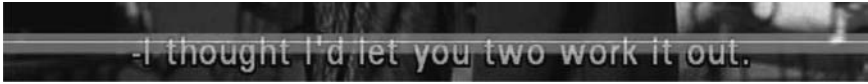
Figure 4.1 The local area for the line in white is highlighted (a total of 11 lines); we use only the information from the local region for text detection and verification. (From Ekin, A., Local information based overlaid text detection by classifier fusion, in Proceedings of the IEEE ICASSP , Toulouse, France, 2006. With permission. Copyright 2006 IEEE.)
