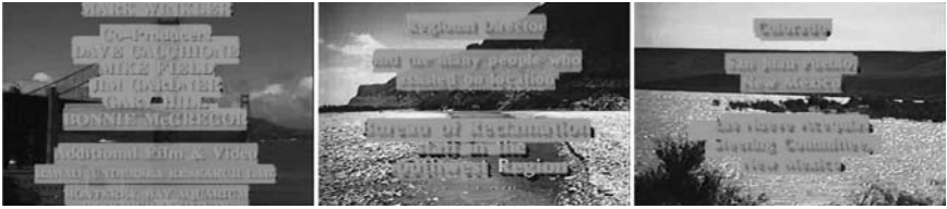
Figure 4.6 The sample results from the text detection algorithm on moving text. (From Ekin, A., Local information based overlaid text detection by classifier fusion, in Proceedings of the IEEE ICASSP , Toulouse, France, 2006. With permission. Copyright 2006 IEEE.)
