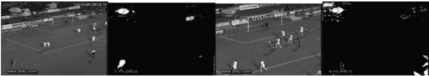
Figure 4.13 A misclassified foreground region in the lower-right corner can be corrected when the detections from other frames are considered. In the scene, only the actual logo region is consistently detected.
