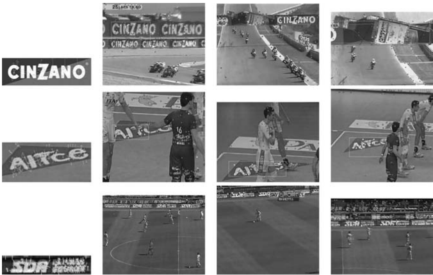
Figure 5.8 Some example matches. The leftmost column contains the trademark model annotated with its detected SIFT feature points. The other three columns contain a portion of a video frame where a match was found. Points indicated in cyan are those selected as “good” matches according to Equations 5.3 and 5.4. (From Bagdanov, A.D. et al., Trademark matching and retrieval in sports video databases , in Proceedings of ACM International Workshop on Multimedia Information Retrieval (MIR) , Augsburg, Bavaria, Germany, 2007. ACM 5/2007, http://www.acm.org/publications/policies/copyright_policy#Retained )
