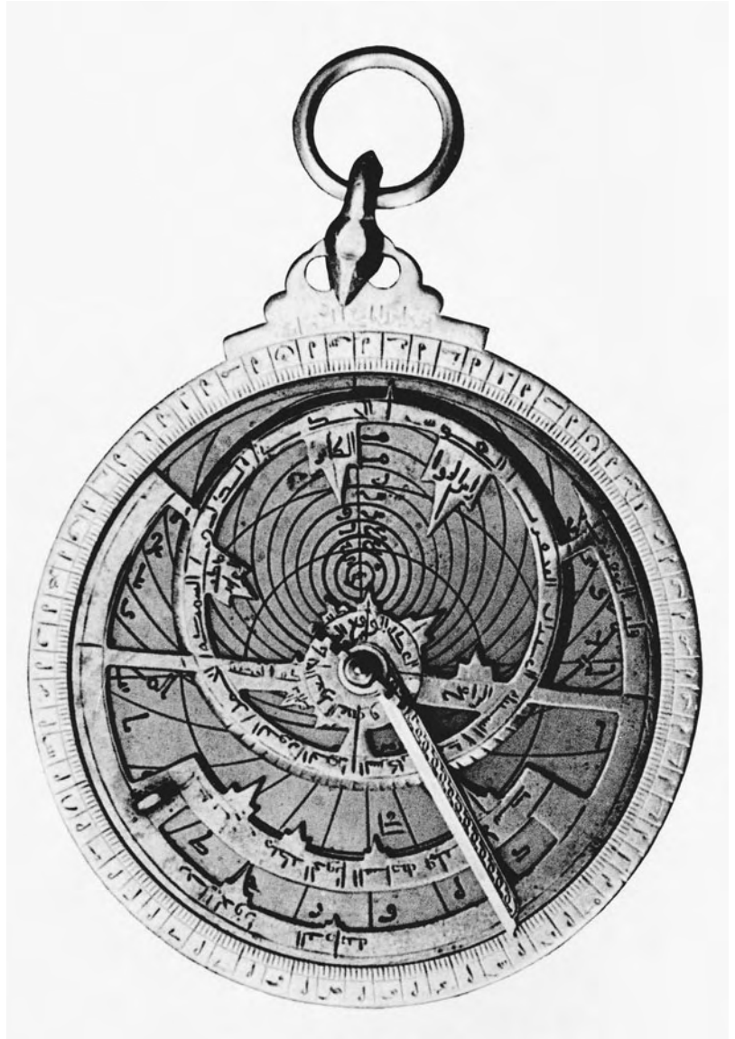
Fig. 6.1. An astrolabe. This multifaceted device was invented in the Islamic world to facilitate astronomical observation and to solve problems relating to timekeeping, geography, and astronomy.
