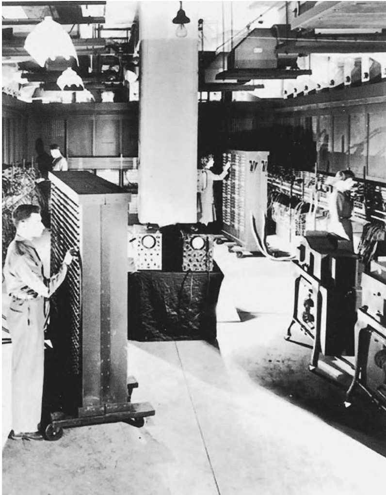
Fig. 19.3. Early computers. An electronic calculating behemoth with 18,000 vacuum tubes, the ENIAC machine (1946) filled a large room and consumed huge amounts of power.
