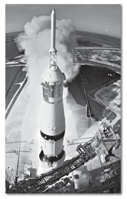
The Apollo 15 spacecraft lifts off from Cape Kennedy, Florida, U.S., atop a Saturn V three-stage rocket, July 26, 1971. A camera mounted at the mobile launch tower's 360-foot (110-m) level recorded this photograph. NASA
