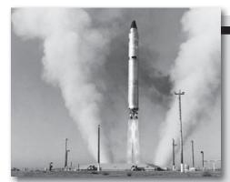
Titan II rocket, lifting off from an underground silo. Developed as an intercontinental ballistic missile, the Titan II also served as a launch vehicle for the Gemini manned spacecraft missions and military and civilian satellites. U.S. Air Force; photograph provided by Donald Boelling
