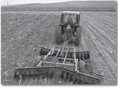
A tractor pulling a disk plow. Courtesy of John Deere
