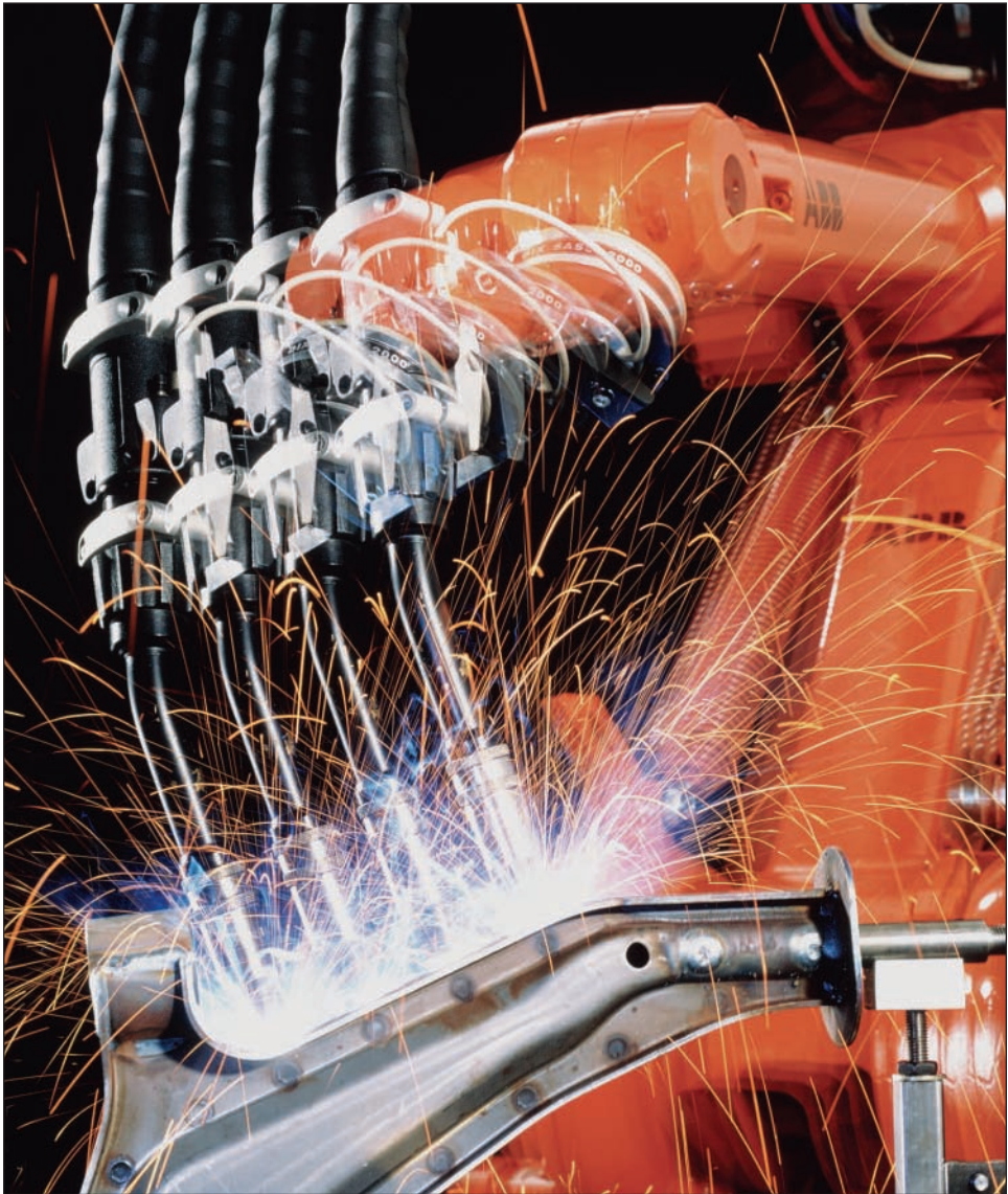
A robotic machine can perform welding operations very precisely, as seen in this multiple exposure photograph.
