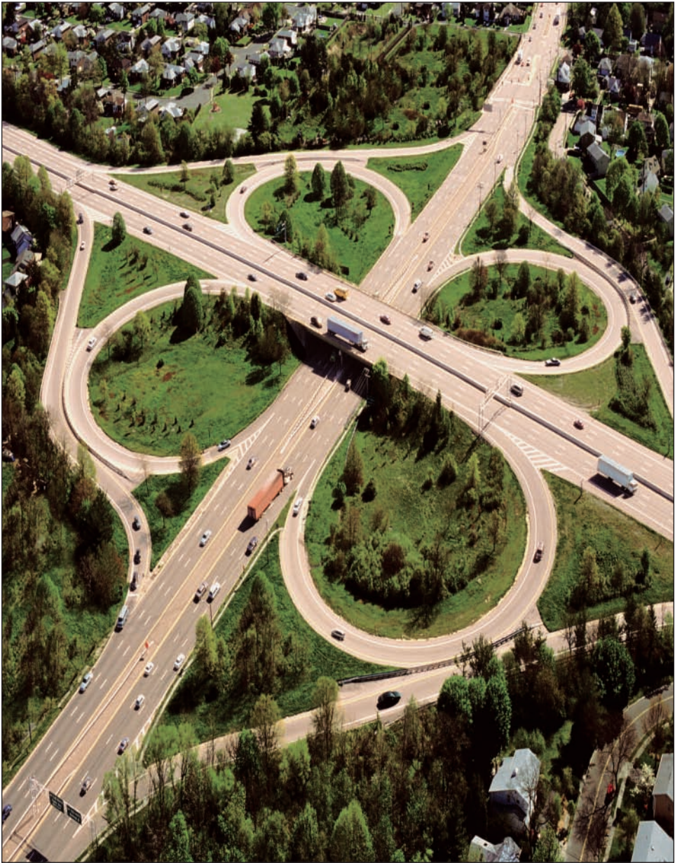
A freeway cloverleaf allows traffic to flow in any direction without stopping, but the design requires a large expanse of land.
