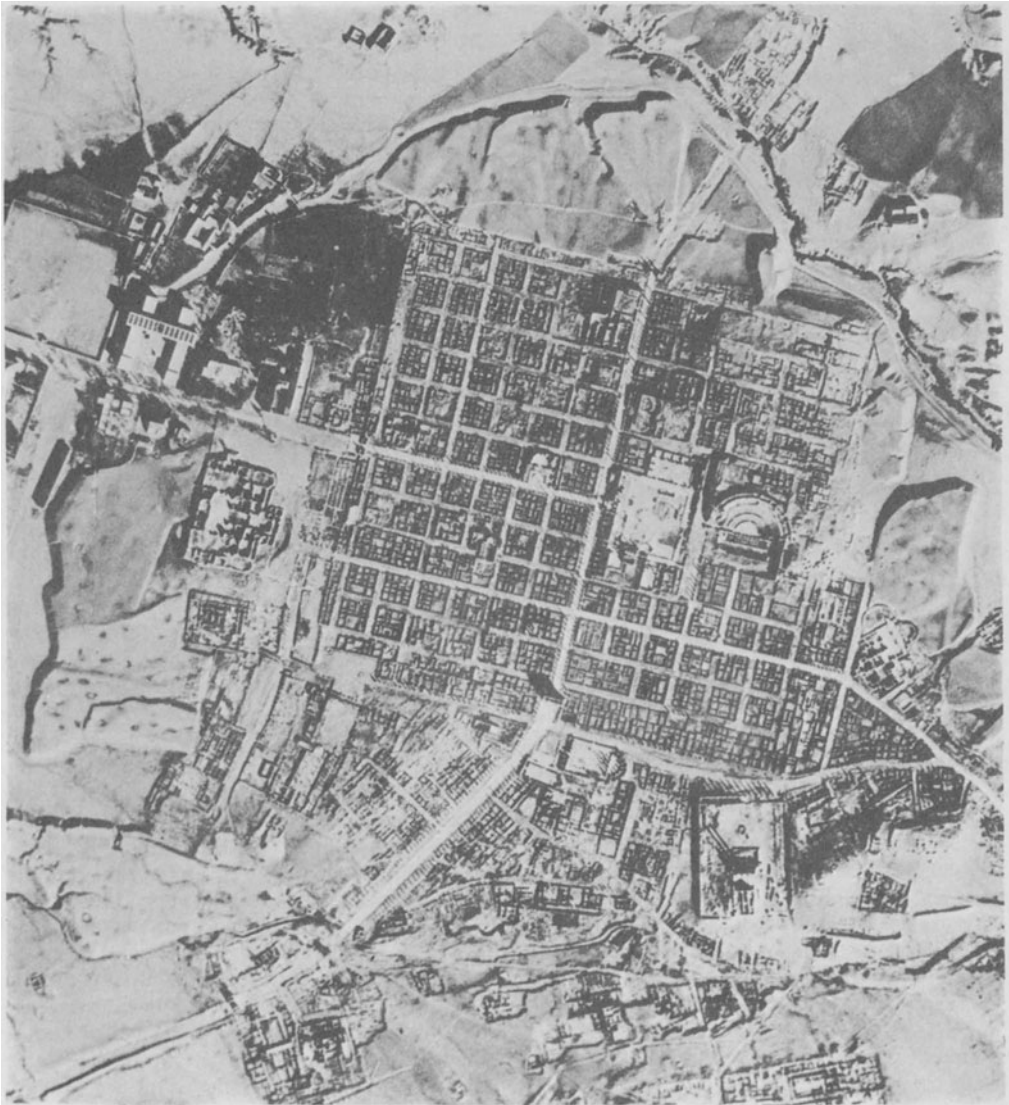
39.16 Air-view of Thamugadi (Timgad). Established by Trajan as a veteran colony, the town was laid out like a camp, with intersecting main streets and grid system. The population c. A.D. 200 is estimated at 12,000–15,000 persons.
