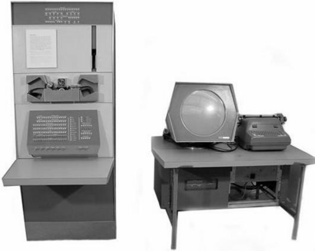
The PDP-1 by Digital Equipment Corporation (DEC). It used punched paper tapes as its primary storage medium and instructions had to be input through a tape reader.
