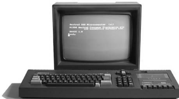
The Z-80 powered CPC 464, the first model in the CPC line. It had 64 KB RAM and an internal cassette deck.
