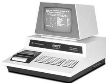
The Commodore PET 2001. It used a MOS 6502 and sold for $795. It was the first computer entirely designed and produced by Commodore.
