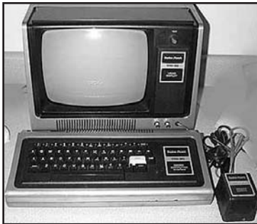
The Tandy/RadioShack TRS-80 Model I, which retailed for $599. Its CPU was a Zilog Z-80.
