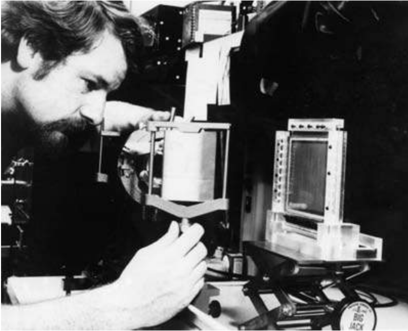
PLATO plasma display panel, circa 1966. Photo courtesy of the University of Illinois at Urbana-Champaign Archives, image 6443.tif.
