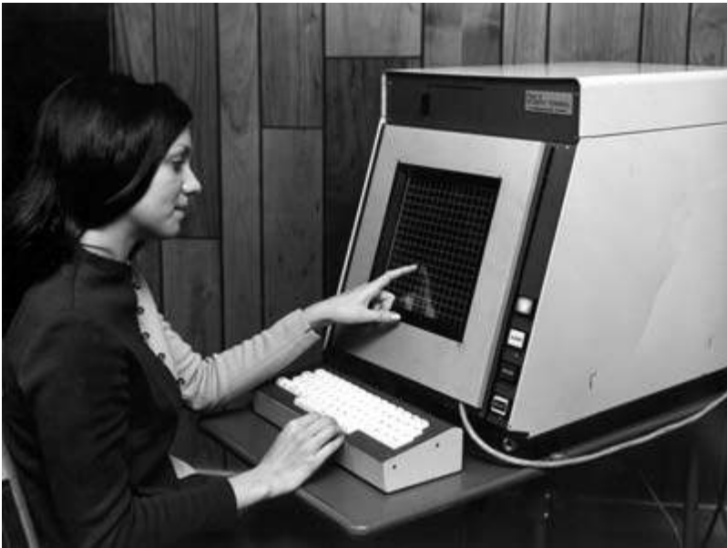
Using a PLATO plasma display terminal, circa 1972–1974. Photo courtesy of the University of Illinois at Urbana-Champaign Archives, image 1141.tif.
