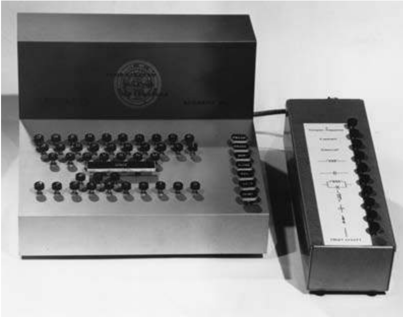
An early PLATO keyset. Note the “AHA!” key in the column of keys on the right side of the keyset, located third from the top. Image courtesy of the Charles Babbage Institute, University of Minnesota Libraries, Minneapolis, Minnesota.
