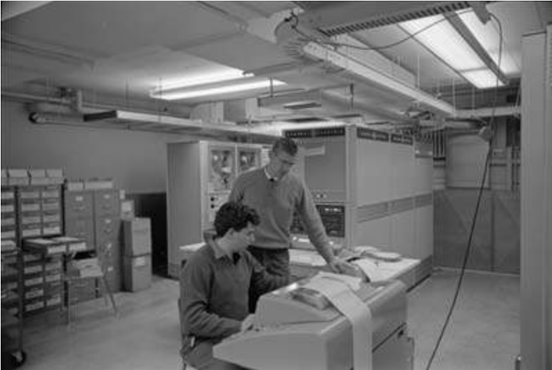
In 1964, Dartmouth College undergraduate Michael Busch ( seated ) worked with mathematics professor Thomas Kurtz ( standing ) to implement the time-sharing system on the GE computer installation in the basement of College Hall. Photo by Adrian N. Bouchard, courtesy of Dartmouth College Library.
